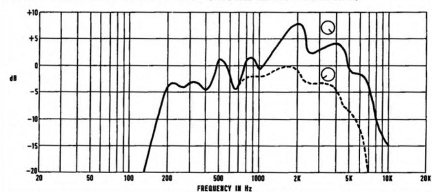
FIG. 6 AKAI X-5 MICROPHONE RESPONSE (700 OHMS IMPEDANCE)
