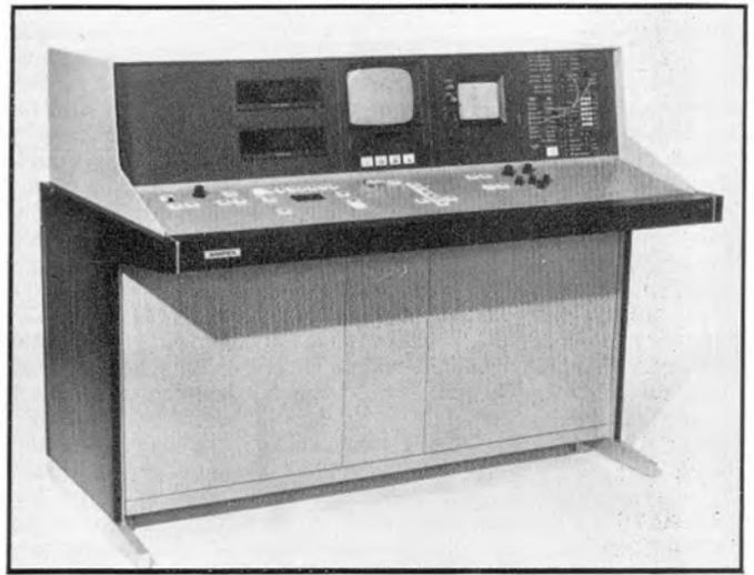
Ampex *HS-200* disc recording and computer-controlled editing system.
