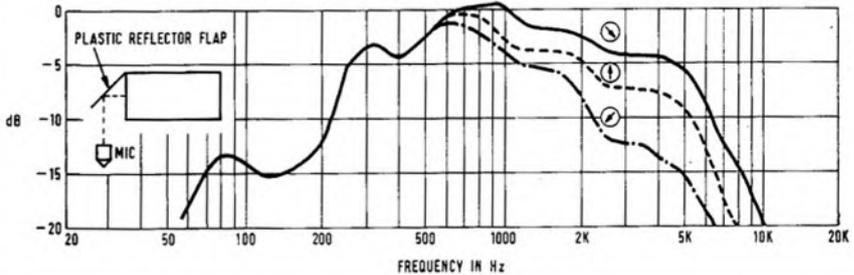
FIG.6 NATIONAL RS-790S MICROPHONE (1K IMPEDANCE)
