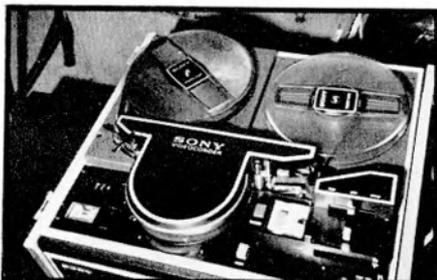
**B** Sony CV2000B, full-track erase head and guides to the left of the video drum.
