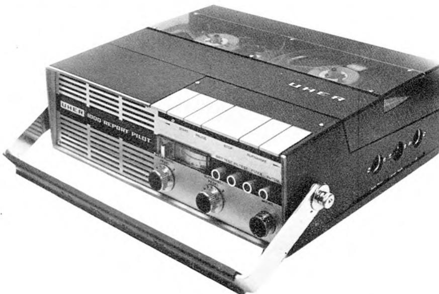
**T**HE Uher 1000 Report Pilot is a self-contained transistor battery portable professional taperecorder developed mainly to meet the requirements of the film industry, with a frame synchronised sound recording pilot-tone system in accordance with DIN standards. It is also useful for 'on the spot' work on account of its light weight and ease of operation.
