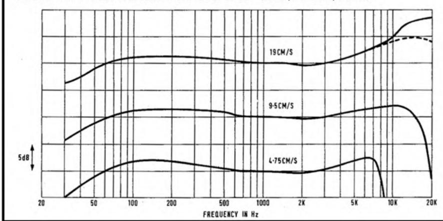
FIG. 6 AKAI X360 ACOUSTIC RESPONSE (WHITE NOISE TEST TAPE TO SOUND OUTPUT)
