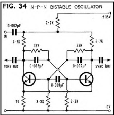
the synchronising signal. Even-order harmonics are wholly absent if the mark-space ratio is 50:50. A much fuller, and variable, harmonic spectrum is obtained by varying this ratio. Such a waveform, by itself, is not sufficient but can be useful, if supplemented by a lower amplitude sawtooth, as a basis for clarinet tone. A square-wave can also be converted to a sawtooth by an integrator circuit (fig. 45 next month).
