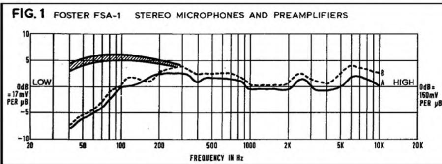
rise from 300 Hz to 30 Hz to give the overall response shown in fig. 1. The overload point is thus increased by 18 dB to 122 dB above threshold, and IEC weighted noise is increased slightly to 42 phons due to the rise in bass response.
