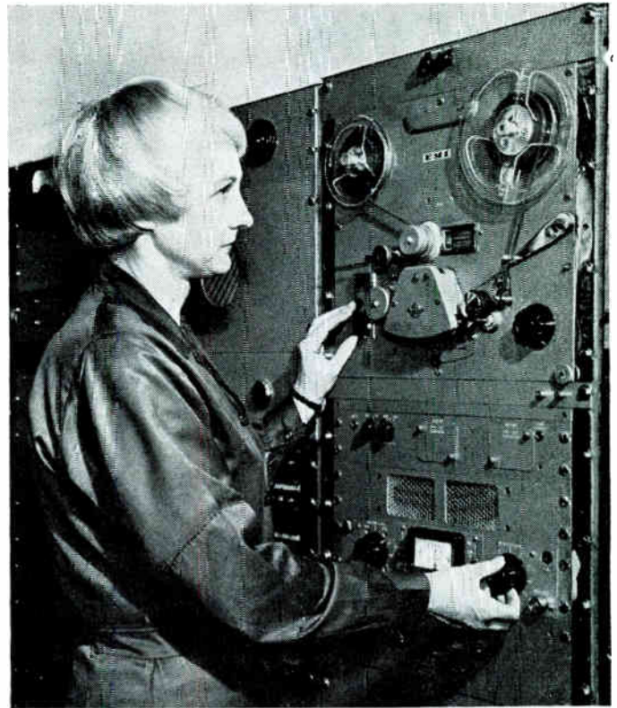
The picture shows an operator at Stagesound Ltd., London, checking the recording before transmission overseas. The recorder is an EMI, TR.90.
