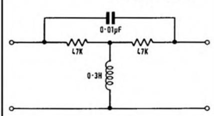
**FIG. 58** TUBA. BASICALLY A BAND-BASS 450Hz LC FILTER FED BY A COMBINATION OF TWO OUTPUTS FROM A FREQUENCY-SENSITIVE VOLTAGE-DIVIDER WITH CLIPPING PROPERTIES.
