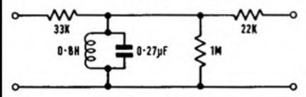
**FIG. 55** TRUMPET. HIGH-PASS RC SECTION FOLLOWED BY LOW-PASS LC TT-SECTION
