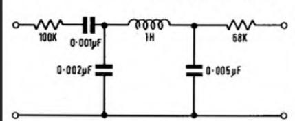
**FIG. 56** TROMBONE. A BRIDGED-T-NETWORK THE BRIDGING LC COMBINATION OFFERS ITS HIGHEST IMPEDANCE (LEAST EFFECT) AT ITS RESONANT FREQUENCY, ALLOWING MAXIMUM SIGNAL VOLTAGE TO BE DEVELOPED ACROSS SHUNT COMBINATION, SIMULATING PRONOUNCED FORMANT.
