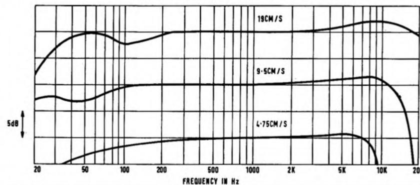
This should be borne in mind when playing prerecorded tapes at 9.5 cm/s into wide-range external amplifiers and speakers. A slight touch of top lift will be required at this speed. If the tapes are played on the machine's own speakers, the treble tone control can be left near the mid setting.
