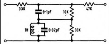
**FIG. 52** BASSOON. A VOLTAGE DIVIDER, OF WHICH THE SHUNT ARM CONSISTS OF A DOUBLE RESONANT FILTER, BOTH SECTIONS BEING DAMPED BY THE 33K RESISTOR. THE SECTIONS RESONATE AT 500Hz AND 1.2KHz
