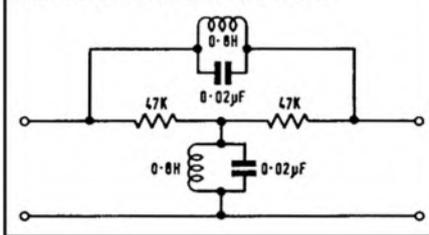
**FIG. 57** SAXOPHONE. HIGH-PASS LR T-SECTION BRIDGED BY A CAPACITOR
