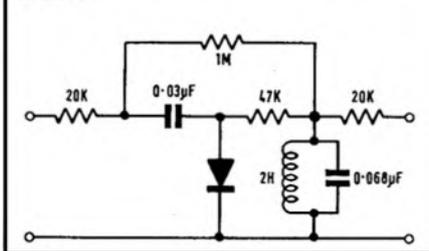
**FIG. 59** VIOLIN. A HIGH-PASS FILTER WITH A LOW TURN-OVER FREQUENCY, FOLLOWED BY A LOW-PASS FILTER WITH A HIGH TURN-OVER FREQUENCY.
