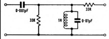
**FIG. 51** CLARINET. A LOW-PASS RC SECTION WITH THE EFFECT OF THE CAPACITOR REDUCED BY SHUNT RESISTANCE, THE EFFECT OF THE L-SECTION BEING FURTHER MODIFIED BY THE INCLUSION OF A DAMPED BAND-PASS FILTER RESONATING AROUND 1KHz
