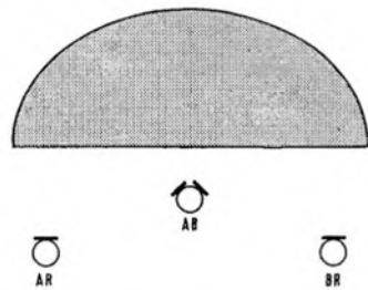
**Fig. 3.** Stereo microphone layout for either 2-channel or 4-channel stereo. In BBC usage AB might be a C12 or a pair of C24's and AR and BR individual C24s. This is one of a range of four microphone (or four-element) layouts which can readily be adapted to the four-channel system.
