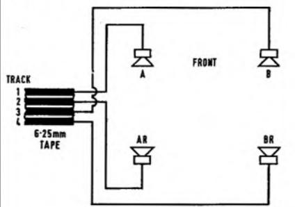
Fig. 2. The Vanguard track configuration for 6.25 mm tape.
