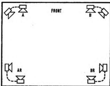
Fig. 1. Four-speaker layout. The arrangement should be symmetrical about a front-to-rear axis, but the rear speakers, AR and BR, need not be opposite the corresponding front speakers, A and B.
