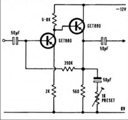
FIG. 11 HIGH GAIN LINE AMP (+84dBm OBTAINABLE)
