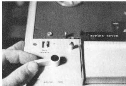
**Fig. 8** (far right) On early models, the function selector tended to work loose. A set of BA Allen keys are an essential for work on this machine. Flattening the spindle may prevent the trouble re-occurring.
