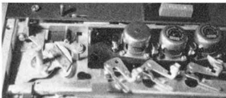
**Fig. 7** (right) The head covers have been removed and lower face plate pivoted up to show the very simple pulley and flap device discussed in the text.
