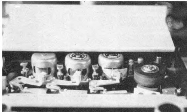
**Fig. 4** Head gate and pressure pad arrangements. Note guide positions.
