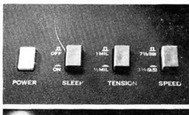
*Pause switch*, *Sleep switch*, *automatically resetting reel clampers*, *responsive pushbutton controls*, and *separate volume controls for two line inputs and another for headphones*.
