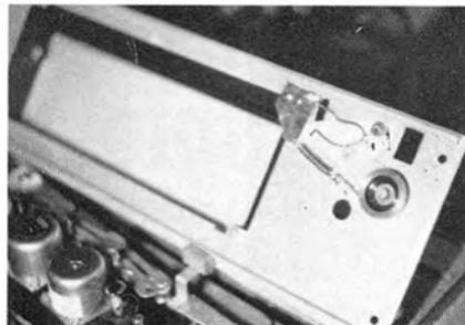
**Fig. 7** (right) The head covers have been removed and lower face plate pivoted up to show the very simple pulley and flap device discussed in the text.
