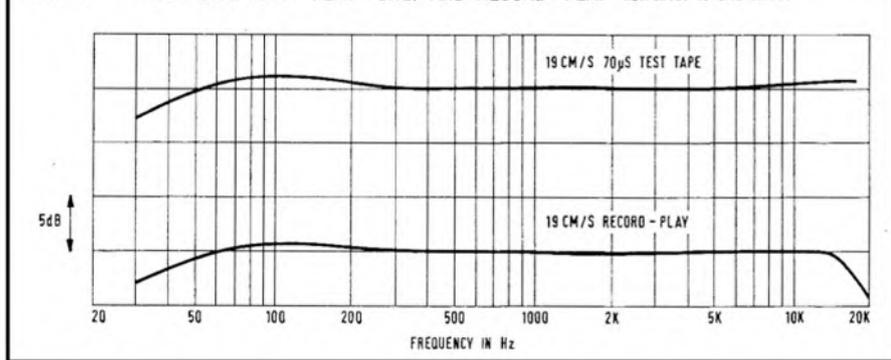
FIG. 3 UHER 1000 MK2 ACOUSTIC RESPONSE LINE IN TO SOUND LEVEL ON LS AXIS
