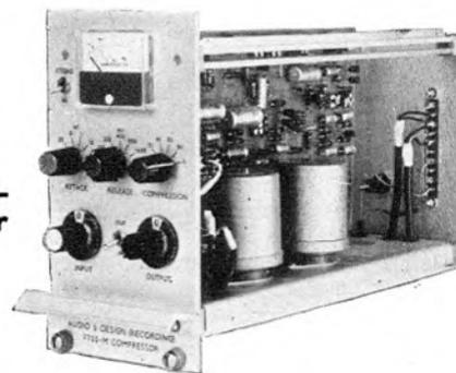
The new F700 Compressor provides a range of compression slopes from less than 2:1 to greater than 25:1; switched attack control for special effects; switched release control from 25mS. The threshold level is switched with compression slope to provide a constant level of output for 17dB reduction. Normal output level (unattenuated) +8dBm. Noise better than -75dB below Limit level Distortion: 0.1% for 25dB reduction.
