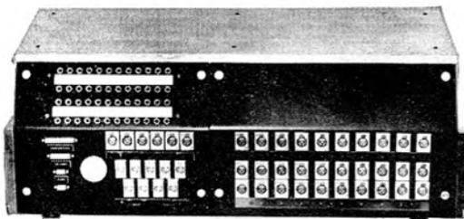
The Neve BCM 10/2 marks a new departure into the field of sophisticated audio control. It embodies ten full mixing input channels and two output groups and is conveniently transportable.
