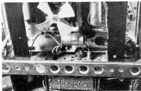
**FIG. 3.** Close-up of the record amplifier board at the chassis side.
