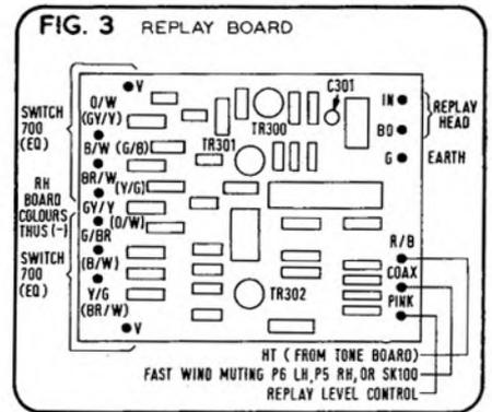
This source reading is incorporated to allow the level of the signal passing through each recording to be selected and indicated regardless of the position of the output switch, which selects the 'off-tape' or 'straight-through' path of the signal. So the meter reads either the replay signal or the source signal, as well as the bias. It needs only the addition of a tone generator in the latest Ferrograph circuitry to bring this development into line with modern studio practice.
