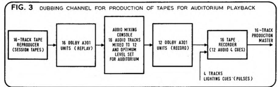
tracks set to match the playback levels on the auditorium stage. At the same time the four tracks containing the chorus were mixed together in pairs with the four tracks containing the ambience and third violins, resulting in a 12-track audio master leaving four tracks available for the pre-programmed lighting cues.
