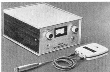
quency specified by the customer. Claimed signal-to-noise ratio is 60 dB. The receiver can be mains or battery powered, typical link range being 10 m indoors and 800 m outdoors.
