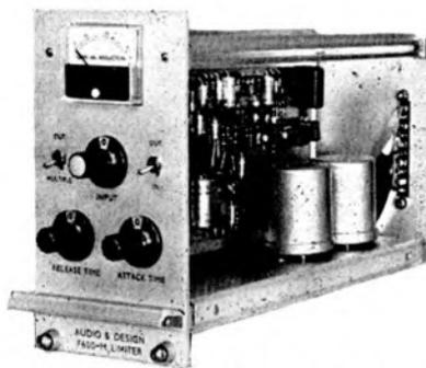
A Mk. 2 version of the well established F600 unit. Gain within the system is normally 25dB with output level of 0dBm (+8dBm to order). Compression ratio better than 25:1; variable attack and release controls with auto network. Noise -70dBm. Response: 10Hz-50kHz for -3dB. Distortion: 0.1% for 25dB reduction at 1kHz.
