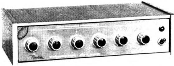
Frequency Response 10 c/s (Hz) to 35 Kc/s (kHz)
