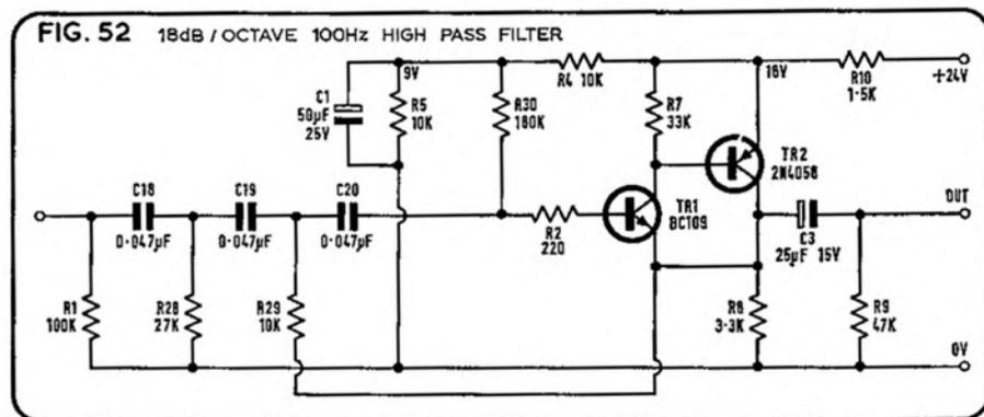
turnover frequencies are shown, but these can be increased in either direction by suitable adjustment of the capacitor values, subject only to physical size and stray capacities. Results obtained with the 3 kHz version were  $-3$  dB at 3.5 kHz,  $-12$  dB at 6.5 Hz, and  $-24$  dB at 13 kHz, which agrees with the theoretical value of 7.3 K for R20 and R21. Use this latter value for any frequency scaling and round off to the nearest preferred value.
