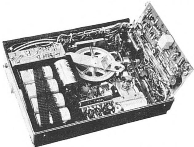
The usual trouble is contact points, and a clearance of 100  $\mu$ m is required. Again, the only adjustment is the bending of the backing strips. I have never found this operation to be entirely satisfactory and avoid it wherever possible. We had a great deal of this to do on older Grundig recorders and used always to carry a stock of spare 'spring sets', finding this more economic than attempting to undo the 'bend and twist' efforts of our predecessors.
