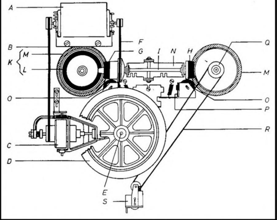
Finally, this month, brakes. From fig. 3 we can see the way the brake rollers O engage with the edge of the turntable. We can also see the shape of the brackets in which these rubber rollers are held, the lever P on which the end-pieces are mounted, and the small springs which aid engagement.
