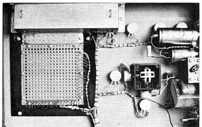
another signal. Two methods of manually controlling *VCS3* circuits have been combined in a joystick, situated to the right of the patchboard. Lateral and vertical movements respectively operate one of two potentiometers, their voltage ranges governed by separate presets. Pins at 15I and 16J would result in lateral stick movement controlling the pitch of oscillator 1, and vertical movements the pitch of oscillator 2.
