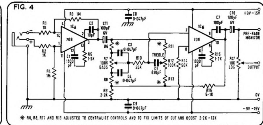
\* R6, R8, R11 AND R13 ADJUSTED TO CENTRALIZE CONTROLS AND TO FIX LIMITS OF CUT AND BOOST 2-2K-12K
