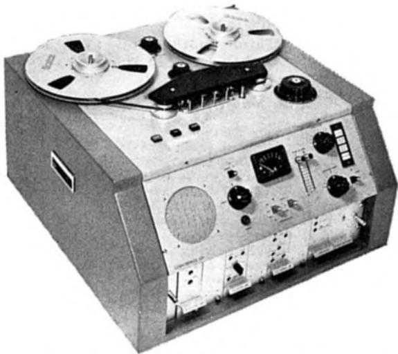
Sensitivity 45 MV for tape modulation of 40 MM per millimetre Line 'Out' 600 Ohms floating. Delivers +8dB across 600 Ohms at maximum level. Up to 16dBm with less than 0.3% distortion
