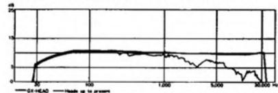
Change in the Characteristics of Frequency Response due to Adhesion of Dust (using tape of inferior quality at 40°C (104°F), 85% humidity)
