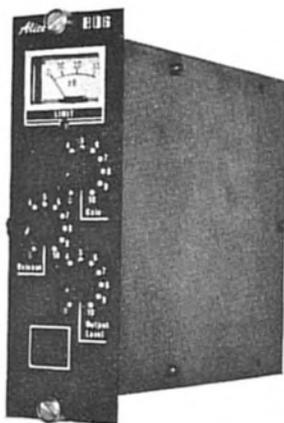
**BD6 LIMITER AMPLIFIER**—A peak limiter with fast attack time and variable release. Limit ratio exceeds 25/1 and overshoot is held to fine limits. Developed for use in a future noise reduction system the circuit is remarkably free of unwanted modulation effects and distortion normally associated with a limiter with this type of action. Input and output nominal 0 dBm balanced or unbalanced. Max gain 16 dB can be supplied in stereo pairs to special order.
