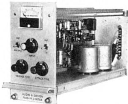
A Mk. 2 version of the well established F600 unit. Gain within the system is normally 25dB with output level of 0dBm (+8dBm to order). Compression ratio better than 25:1; variable attack and release controls with auto network. Noise—70dBm. Response: 10Hz—50kHz for -3dB. Distortion: 0.1% for 25dB reduction at 1kHz.
