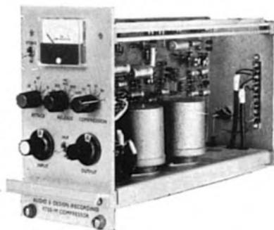
The new F700 Compressor provides a range of compression slopes from less than 2:1 to greater than 25:1; switched attack control for special effects; switched release control from 25mS. The threshold level is switched with compression slope to provide a constant level of output for 17dB reduction. Normal output level (unattenuated) +8dBm. Noise better than -75dB below Limit level Distortion: 0.1% for 25dB reduction.
