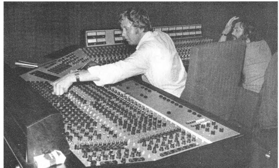
Each microphone channel also has 'prefade listen' and 'check' function. The check switch provides a very useful function, when in the check position, of turning all the other modules in that section of the desk off.
