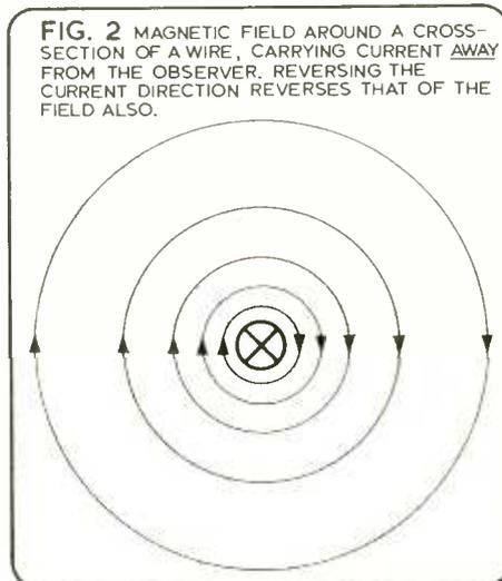
FIG. 2 MAGNETIC FIELD AROUND A CROSS-SECTION OF A WIRE, CARRYING CURRENT AWAY FROM THE OBSERVER. REVERSING THE CURRENT DIRECTION REVERSES THAT OF THE FIELD ALSO.
