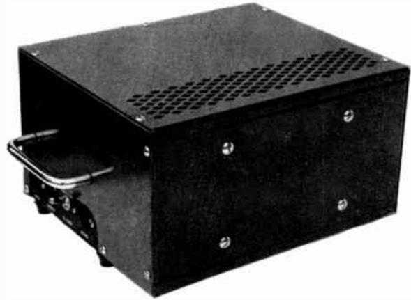
Outputs are for 8 ohms/15 ohms OR 100 volt line. Gain control extra if required. The input required is less than 0.5 volt on 100K ohms. Weight 28lb. Size  $12'' \times 6\frac{1}{2}'' \times 9''$ .
