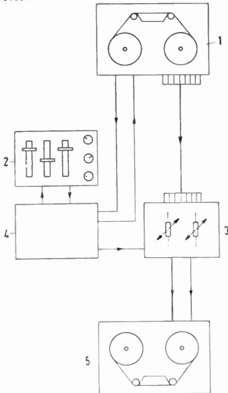
record the individual acoustic events. The seven audio tracks on machine 1 are subsequently copied on to machine 5 through servo elements 3. Electronic or electromechanical elements may be employed, following the control settings determined during the original mix. If amendments are required at this stage, the control track read/write head is switched to write again and the mixer 2 adjusted to produce new control signals for the servo elements.
