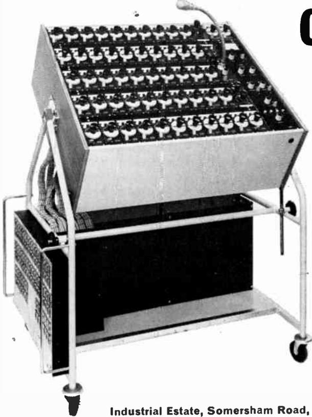
The photograph shows the 50-way trolley-mounted console of a complete sound distribution and mixing system recently completed to special order. Ideal for either studio or location work, it operates either from mains or 12 volt battery and incorporates a jack field and two integral 30 watt power amplifiers.
