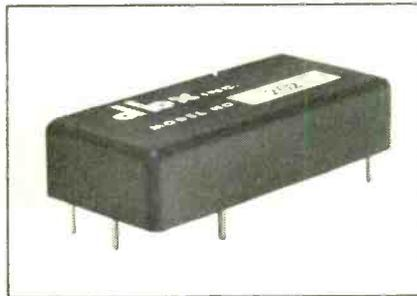
**Model 202**, linear dB gain vs: control voltage, -100 to +30 dB gain, noise 130 dB below peak level, low distortion.
