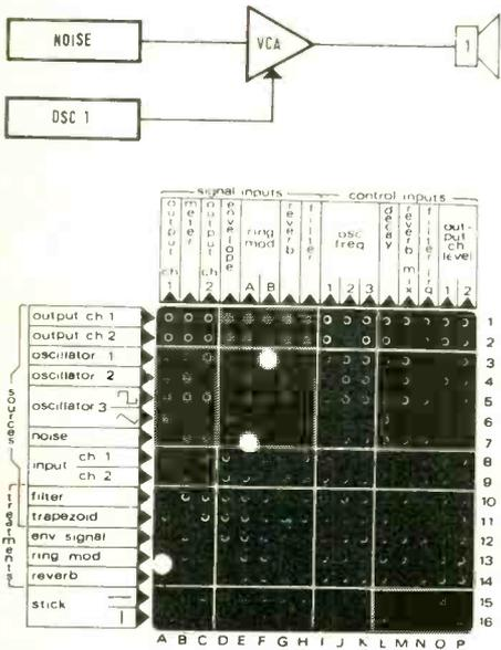
to input A of the ring modulator. A second pin at 3F routes the output of oscillator One to input B. Setting a 1 Hz sinewave from oscillator One (fig. 5), the vca integrates this with the noise signal to produce a 1 Hz rise and fall in noise amplitude: a very approximate steam engine. Tones may be similarly interacted, perhaps the greatest value of the ring modulator being its ability to produce relatively complex waveforms from the three basic shapes generated by the oscillators.
