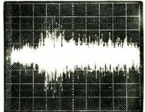
FIG. 5 20 ms/div white decay reverberation characteristic
