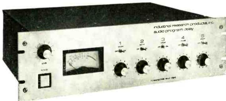
The Audio Program Delay (DA 4003) offers up to five outputs from a single input with time delays up to 240 milliseconds. Delay steps of 10 milliseconds are standard and are selected with panel mounted switches. The versatility of delay selection with multiple outputs gives the professional recording artist an opportunity to produce a variety of sound colouring effects.
