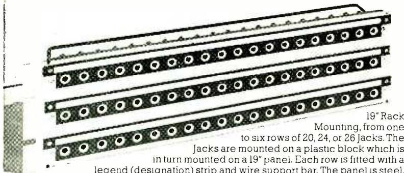
19" Rack Mounting, from one to six rows of 20, 24, or 26 jacks. The jacks are mounted on a plastic block which is in turn mounted on a 19" panel. Each row is fitted with a legend (designation) strip and wire support bar. The panel is steel, cadmium plated, chromate passivated and stove enamelled hammer tone silver.
