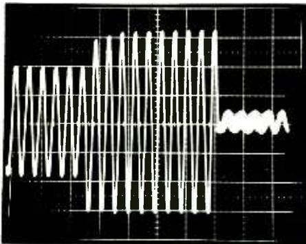
FIG. 2 1 kHz 10 ms burst +18 dB limiting
