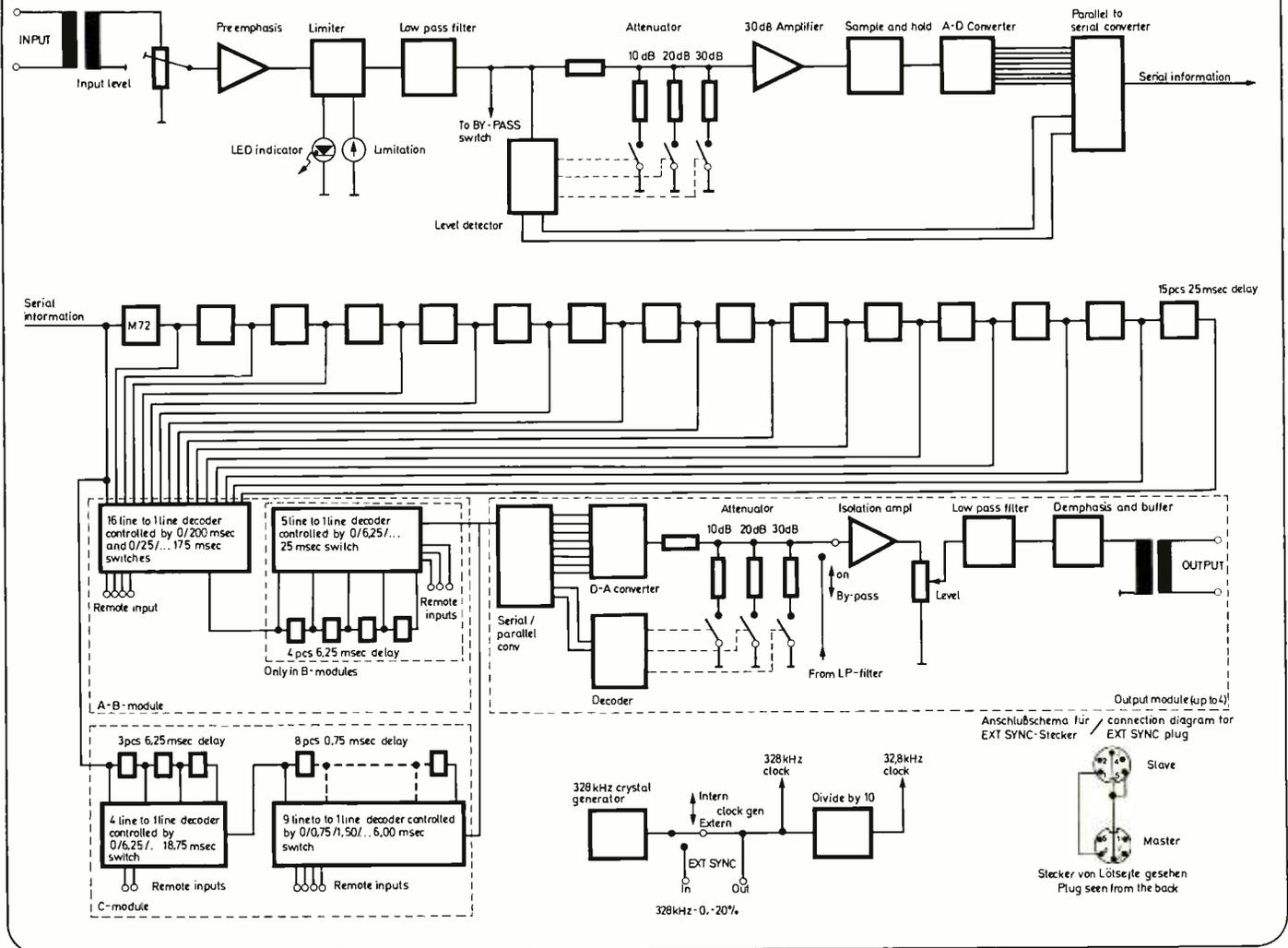
containing two printed boards. The type 72/1 module which was supplied with the review sample has four front panel controls. One of these is a miniature toggle switch providing for bypass of the digital section of the delay unit, but leaves the filters, pre- and de-emphasis and the 'limiter' in action in the bypass mode.
