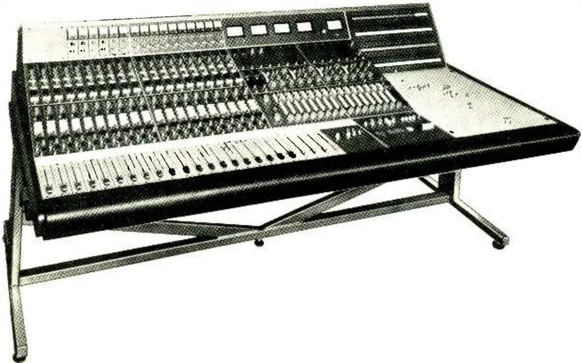
The Neve way to real economy is the 8034. It is a flexible sound mixing console that has all the facilities for a modern studio working with up to 16 track techniques on original recording or for multi-track reduction.
