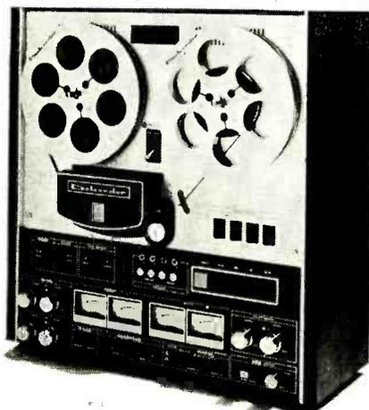
Similar facilities to Teac 3340. Three motors, 3 heads, solenoid operation, electronic echo. Speeds 7½ and 3¾ i.p.s., 7in. spools. Mic and linemixing.
