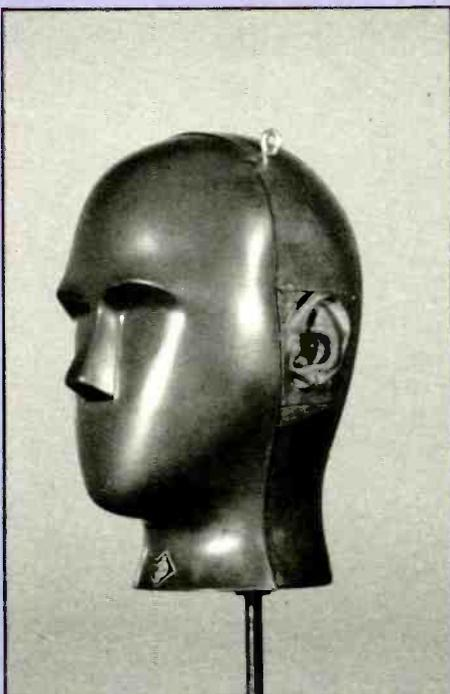
Going under the name of *KU 81* the latest dummy head developed by Neumann contains two capacitor mic amps. The ear is made of material which has very similar mechanical properties to human flesh
