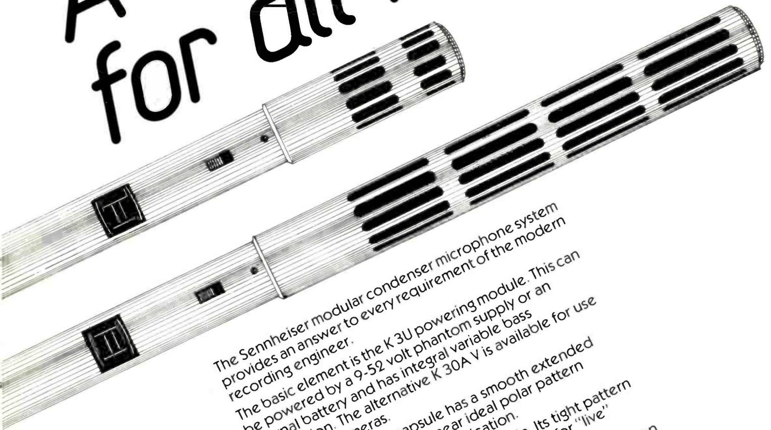
The Sennheiser modular condenser microphone system provides an answer to every requirement of the modern recording engineer. The basic element is the K 3U powering module. This can be powered by a 9-52 volt phantom supply or an internal battery and has integral variable bass attenuation. The alternative K 30A V is available for use with video cameras.
