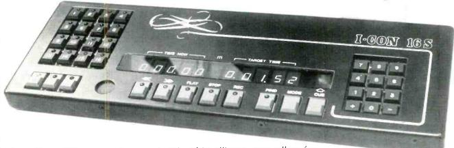
The I-CON 16S is one of a new family of intelligent controllers for audio tape and video which includes not only all the autolocate functions of the CM50 but also a choice of 16 or 24 track select keys with a serial data link to the tape deck (we provide the decoder). The 'S' suffix means that the I-CON may also be equipped as a simple synchroniser for some tape machines (including the B16 and Tascam 58).
