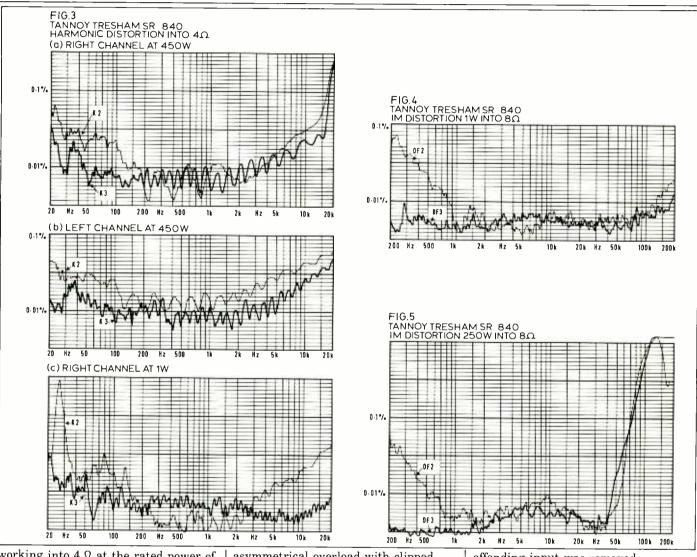
working into  $4 \Omega$  at the rated power of 450 W and at 1 W, and found to differ for the two channels, particularly at 450 W. These results are shown in Figs 3a and 3b. Smaller differences occurred at 1 W with Fig 3c being typical.
