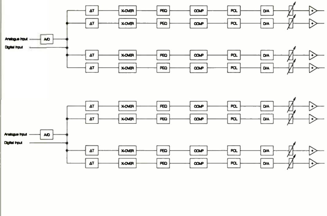
Fig.20: Block schematic for Yamaha D2040
