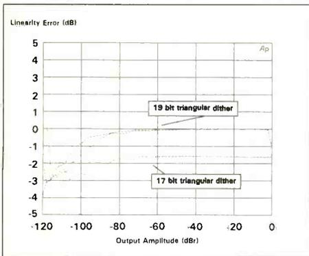
**Fig.9: D-A convertor linearity error — note variation with dither level. Curves are offset for clarity**
