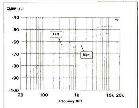
Fig.4: Input Common Mode Rejection Ratio
