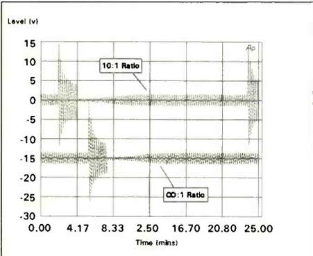
Fig. 19: Compressor-limiter dynamic characteristics. Threshold +5, attack time 1.0ms, release time 0.015
