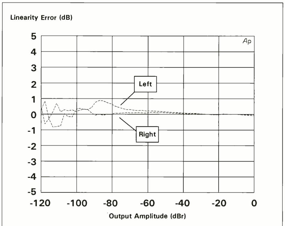
Fig.8: A-D plus D-A convertor linearity error
