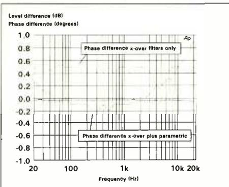
Fig.6: Phase and level difference, single channel left and right outputs. Crossover 800Hz and 5kHz, 24dB/oct slopes parametric equalisers: +6dB at 1.6kHz, Q=1 and -6dB at 3.2kHz, Q=7
