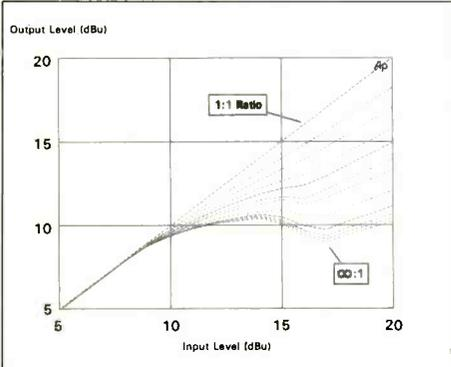
Fig. 18: Compressor-limiter—effect of ratio variation
