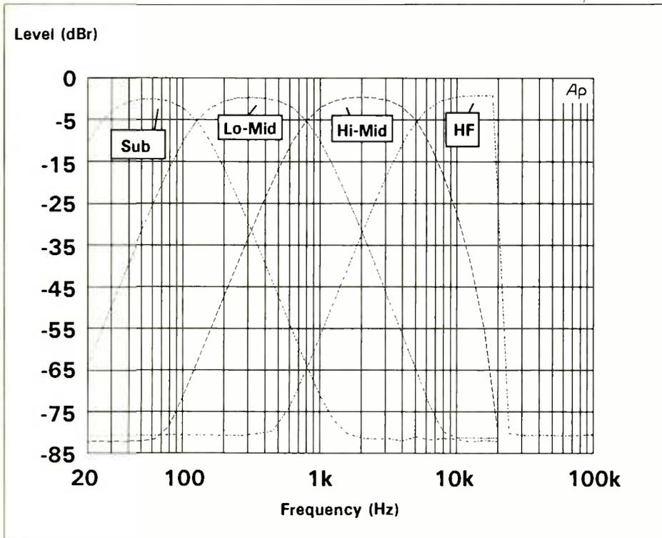
Fig.1: Typical four-way crossover characteristics
