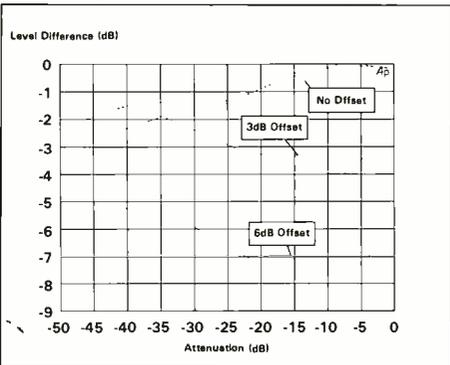
Fig.7: Tracking of output level attenuators
