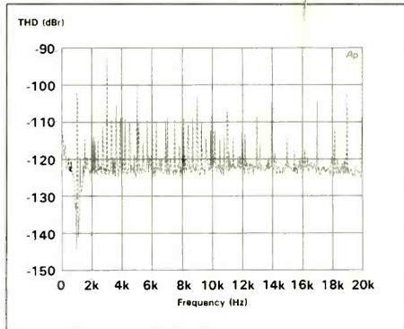
**Fig.15: THD Spectrum with 997Hz analogue stimulus at +20dBu. Note modulation noise products when A-D is in use**
