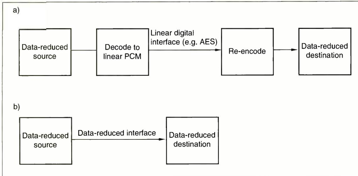
**Fig.1: At (a) the data reduced source is decoded to linear PCM before being transferred via a conventional interface, and quality will be affected. At (b) the data reduced information is transferred without reconverting to linear PCM and no quality is lost**
