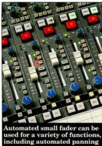
Automated small fader can be used for a variety of functions, including automated panning
