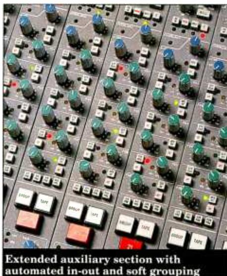
Extended auxiliary section with automated in-out and soft grouping
