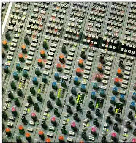
**SL 9000j series 48-track routing selectors and improved dynamics section**
