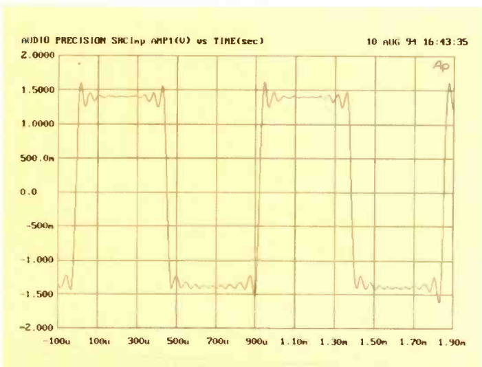
Fig.3: Square-wave response for 7% sample-rate increase through AD 1890
