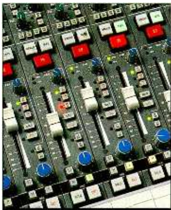
Automated small fader can be used for a variety of functions, including automated panning
