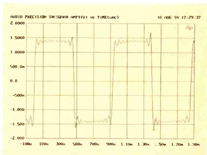
Fig.4: Square-wave response for 7% sample-rate increase through Motorola 5501
