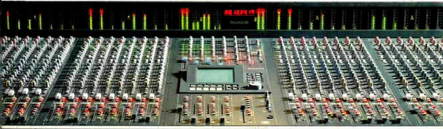
control of up to eight D2040s which may be configured as a number of subgroups and controlled accordingly including such facilities as labelling, muting and soloing 'in place'. Control data may be recorded, edited and saved to disk allowing transfer of control between systems.
