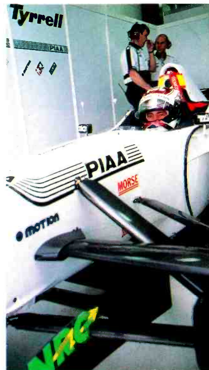
Camera mounting impinges on aerodynamic efficiency
