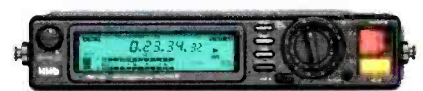
PDR1000 4 head, 4 motor portable professional DAT recorder with 44.1/48/32kHz recording, balanced XLR analogue I/O and AES/EBU + SPDIF digital I/Os.
