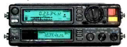
PDR1000TC 4 head, 4 motor professional portable DAT recorder equipped to record, generate and reference to timecode in all existing international standards.
