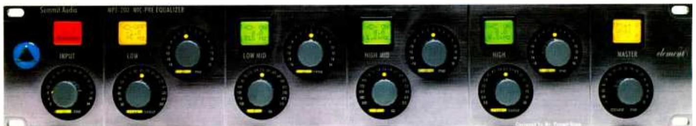
selects the section to be on (green) or off (amber). The turnover frequency is indicated in the screen and for the low and high sections, pushing the FREQUENCY knob changes the characteristics from peaking to shelving. In the case of the mid sections, pushing the knob calls up the Q function which can be varied between 0.6—2. For all sections, pushing the BOOST-CUT control selects Coarse or Fine settings, with Coarse being 2dB steps and Fine 0.5dB steps.
