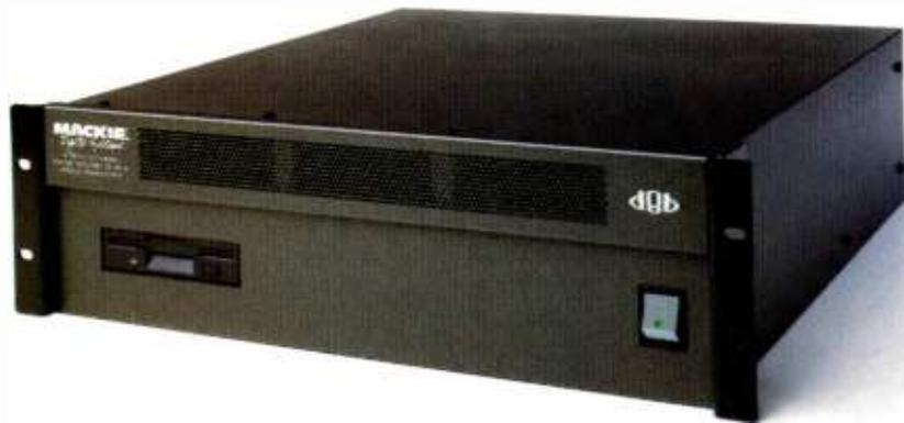
◀ job of disguising the PC. It runs MackieOS which presents a GUI to the operator but manages to avoid most of the complexities of Macs or Windows. The cooling fan makes an infernal din so the (approx) 5m cables may seem less than generous when it comes to remote siting.
