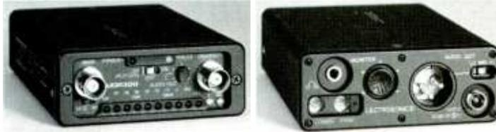
in the transmitter and a de-emphasis HF roll-off in the receiver, that in conventional systems can provide an improvement in signal-to-noise ratio of up to 10dB, providing the two halves are perfectly matched; if they are not, this again results in an altered signal from the original; the dual-band compander of the Lectro provides its own dynamic pre- and de-emphasis function.
