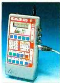
**Prism Sound** produces the DSA-1 hand-held AES/EBU analyzer, the Dscope FFT analyzer and high-quality A/D and D/A converters. The DSA-1 is the only hand-held tool that measures carrier parameters and data content. With programmable
