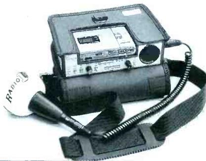
The Carrier is a simpler and cheaper version of the MobiDisc and is similarly built around a MZ-R30 machine. It features a mono (or stereo) XLR mic input, a stereo cinch line output and a 1/4-inch stereo jack headphone output.
