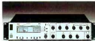
reduction metering. It offers variable soft knee, programme dependent release, oversampling side chain and gain multiplier, an auto gain makeup feature.
