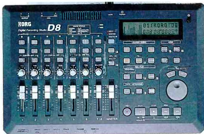
The D8 8-track hard-disk recorder has a 12-channel 4-bus digital mixer incorporated together with a 1.4Gb drive.
