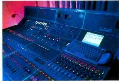
The Digital T Series console combines the assignable control surface of the established T Series mixing system with an all-digital signal path. Aimed at on-air
