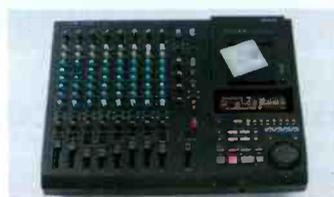
punch in and out with 99 takes, song edit, and cue with a shuttle dial. The recorder is has an 8-channel analogue mixer with 3-band EQ, 2 auxes, pans and faders.
