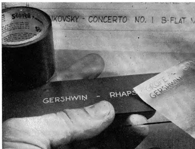
The plastic binding material is adhered to a piece of glass then the gold embossing paper and lettering taped over it so they cannot shift. After tracing the lettering they are removed as shown.
