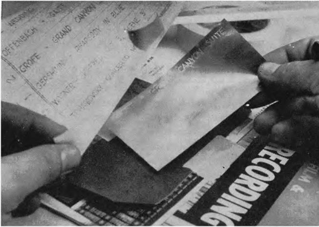
First do your lettering on a piece of tracing paper. The binding material, gold foil and tracing paper are then taped in position on a piece of glass and the lettering traced with a ball-point pen.
