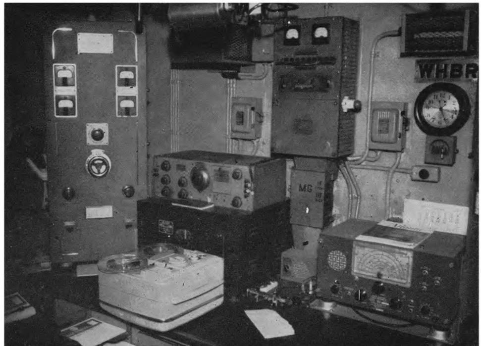
The radio room of the Thompson Lykes with a Revere TR-1200 set up to record. With a recorder in the radio room the operator can meet emergencies by taping one frequency while listening on another.
