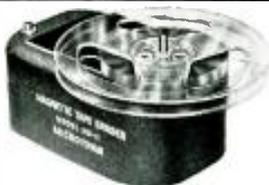
Erases recorded signals and noise from magnetic tape without rewinding. Spindle mounting of reel permits rapid coverage without missed spots. Noise level reduced below level of standard erase heads. Restores tape to like new condition or better. Reel size range 5", 7", 10½". May also be used for demagnetizing record—playback—erase heads.
