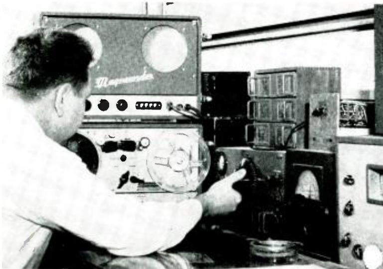
Melvin Hastings tunes the HRO receiver on 20.005 megacycles to catch the beep, beep signals from the Russian satellite sputnik. The output from the radio receiver was fed into the Magne-corder shown and results of the recording were excellent. At one point the signal was picked up while the satellite was 3,000 miles from the station. When almost overhead the signal from the one watt transmitter on the satellite was so loud volume had to be turned down for recording.
