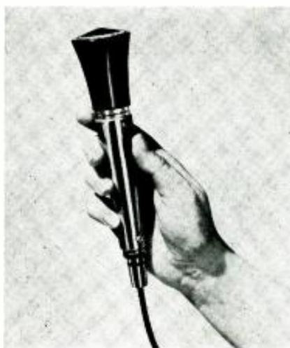
Shure Brothers, Inc., 222 Hartrey Ave., Evanston, Ill., has introduced a new microphone series, the Commando. The Model 430, shown above, is a dual impedance unit featuring an on-off switch and a swivel adapter. The microphone is of impact-resistant plastic, the handle of die-cut zinc, and the Commando can be used in the hand or on a floor or desk. It is available also in a Lavalier model and a Standard model. It is priced at \$38.50. Contact Shure for complete details.
