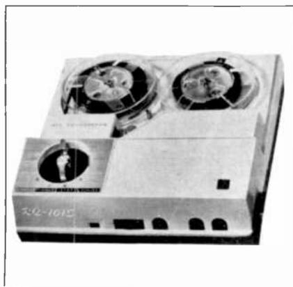
To outward appearances, this machine is very ordinary; it looks more or less like most Japanese transistor recorders. But the similarity ends there. This compact two-hands full has a positive capstan drive and two speeds— $3\frac{3}{4}$  and  $1\frac{7}{8}$  imps. The capstan is covered by a removable drum whose larger diameter provides the faster speed. Changing speeds is relatively easy,
