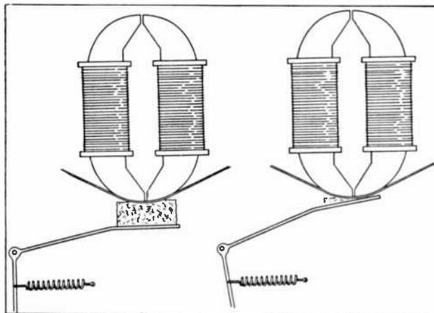
*Above is typical record head. Note narrow gap. At right is same head when badly worn. Note that constant wear and abrasion has worn away the narrow gap, destroying high frequency response and increasing signal-to-noise ratio.*
