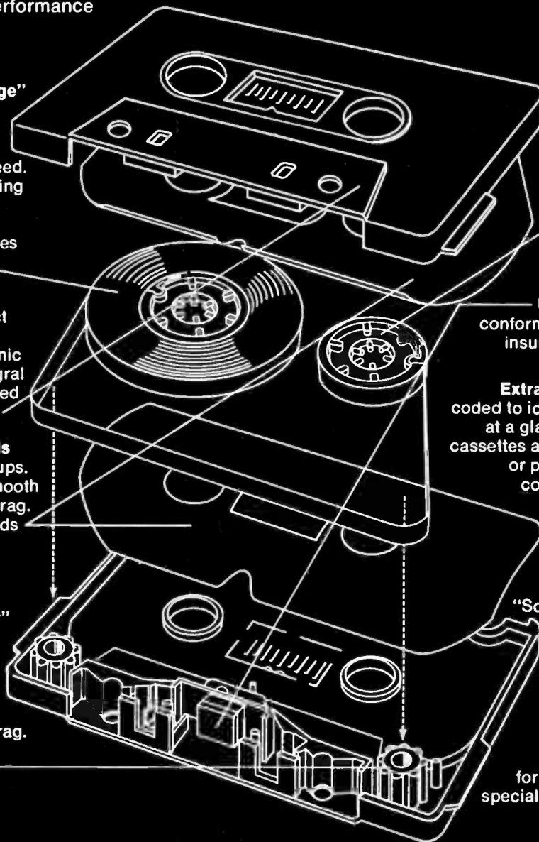
**One-piece hub** locks leader tape securely, eliminates "bump" that can distort tape in winding.
