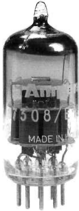
1970s Amperex PQ 7308/E188CC (high quality 6DJ8)
