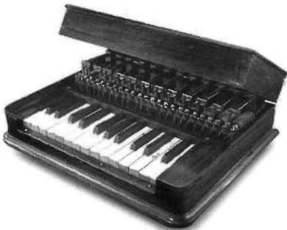
Fig. 1. Elisha Gray's musical telegraph, used in traveling exhibitions to demonstrate his multiplex system (1876).
