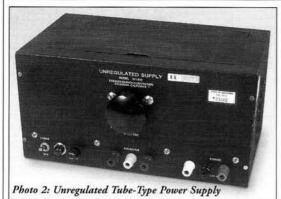
high-voltage transformer driven by a variac. A filament transformer wired ahead of the variac supplies the 5 volts for the rectifiers as well as 6.3 volts to the front panel.
