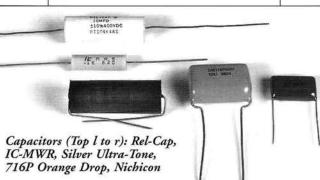
the 716P polypropylene film and aluminum foil with solid copper leads. Sonic qualities of Orange Drops depend on the application. In hi-fi coupling stages, they can have a tubby bass response and somewhat smeared highs. However, the midfrequencies can be big and musical. This can work well in guitar amplifiers and in certain hi-fi applications.
