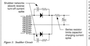
area. This current spike contains a large amount of high-frequency energy. This can shock-excite any parasitic tuned circuits in the transformer or wiring. All this high-frequency energy can get into sensitive circuitry. This problem is most acute when the rectifier is drawing current when the voltage across it reverses, so is especially troublesome in choke-input circuits.
