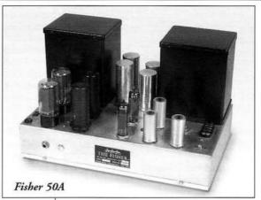
connecting the EL34s in triode, beefing up the power supply and replacing the selenium rectifier with a fast recovery diode.
