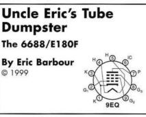
For obvious reasons, the hard core of tube DIYers has started to use hightransconductance frame grid tubes for small-signal gain. Although they can vary in linearity, just as more conventional small-signal types do, frame grids offer low plate resistance and (hopefully) lower microphony.
