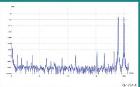
19kHz + 20kHz intermodulation signal
