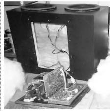
PHOTO 2: Twin subwoofer, with amplifier module in foreground.
