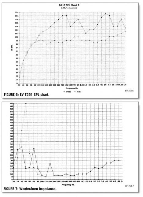
the mids and highs, the renowned  $EV^{TM}$  T251. It is close to the DR10 in size (about 7ft<sup>3</sup>), though at 78 lbs, it weighs over half again as much. Typical of commercial cabinets, it has an average SPL of 98dB.
