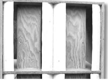
PHOTO 18: Chamfering quartered PVC on the jig.
