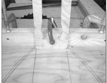
PHOTO 11: Attaching the tweeter baffle to the top using a guideboard for accuracy.
