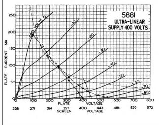
**FIGURE 9: Tube** characteristics for ultralinear operation with a supply of 400V (plate or screen to cathode). The curves were plotted by reducing the screen voltage from 400 by 43% of the reduction used for the plate (increase same way). Composite and individual load lines are also shown, as for triode and pentode operation.
