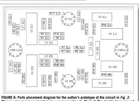
This is a top (component side) view corresponding to Photo 2. The double lines around three sides of the board show the location of the copper ground wire underneath the board (see Photo 3). G-1688-6
