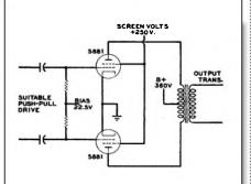
FIGURE 5: Schematic of output circuit, using 5881 tubes as tetrodes (commonly called pentodes, because of the similarity of the operating characteristics). put, will give a corresponding amount of feedback. What offsets this fact is the high plate resistance of the pentode, which means that a much larger amount of feedback must be used to obtain a satisfactory damping factor.
