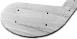
PHOTO 19: Cut and drilled top. www.audioXpress.com
