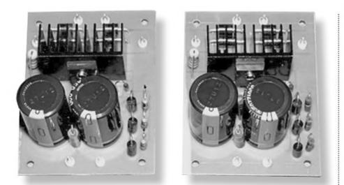
PHOTO 4: The MOSFET and Zener Diode Ripple Filter.
