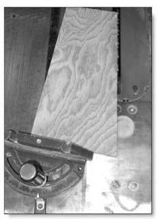
PHOTO 5: Cutting angled piece of plywood to modify panel cutting jig.
