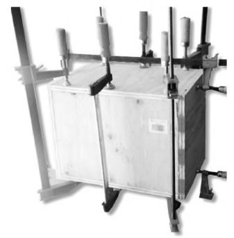
**PHOTO 1: The box glued and thoroughly clamped. 82** audioXpress 1/01
