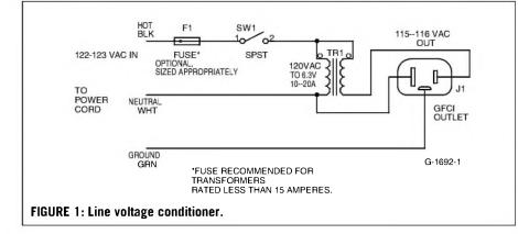
mend that you use a fuse if your filament transformer is rated for less than 15A since you can't expect your home's 15A circuit breaker to protect it. You could also add electrical noise filters and a neon lamp wired to the GFCI receptacle.
