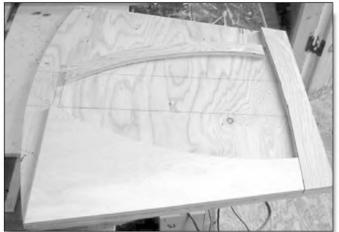
PHOTO 7: Checking brace patterns against cabinet top.
