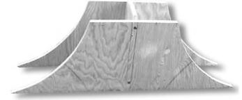
PHOTO 8: The throat horn sides and throat divider assembled.
