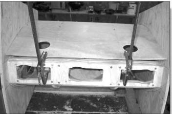
PHOTO 15: Attaching the mouth horn sheathing.
