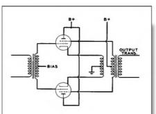
FIGURE 10: Schematic of circuit for operating tubes as ultralinear cathode followers. For 43% equivalent tapping, the screen winding must have 57% of the turns in the cathode winding. Extremely good coupling between the cathode and screen windings is essential.
