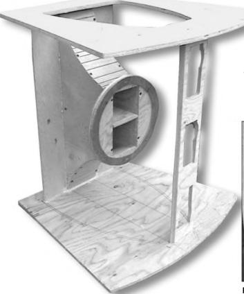
PHOTO 12: Assembly prior to horn brace installation. rate  $80^{\circ}$  cuts (or  $100^{\circ}$ , depending on point of view), instead of the usual  $90^{\circ}$ . Doing this on a table saw is easy if you first cut two pieces of scrap plywood at a  $10^{\circ}$  angle, using your miter gauge (*Fhoto 5*). Screw these directly to your panel-cutting jig (if you haven't yet made one, do it now), allowing you to feed a panel across the saw table at a perfect  $80^{\circ}$  angle (*Fhoto 6*).
