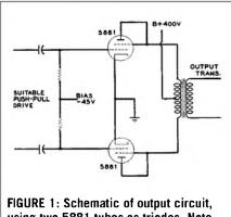
FIGURE 1: Schematic of output circuit, using two 5881 tubes as triodes. Note that screens are connected to plates.
