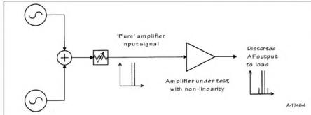
FIGURE 4: Producing multi-tone test signals with standard sinewave signal generators. Harmonic output of the generators is not critical. The passive combiner and attenuator should not affect the measurement linearity—their IP3 can be measured in principle by increasing the generator output level beyond what the amplifier requires, allowing the effective generator IMD to be calculated at the lower levels for the amplifier test.
