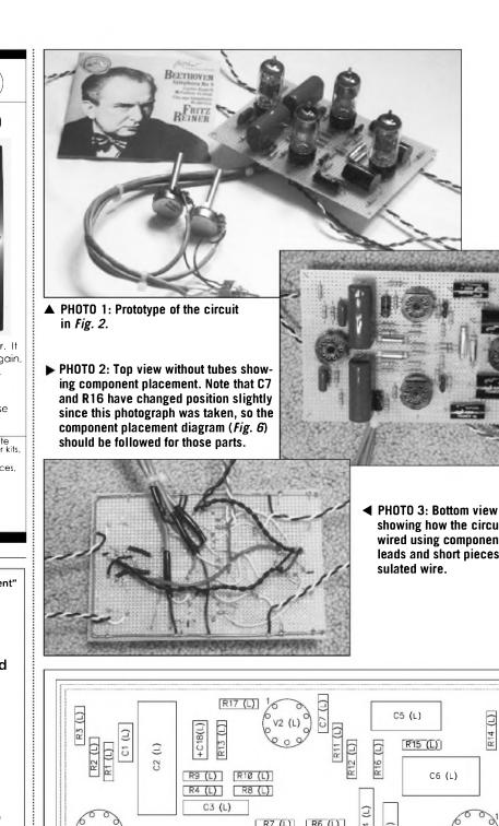
showing how the circuit is wired using component leads and short pieces of in-
