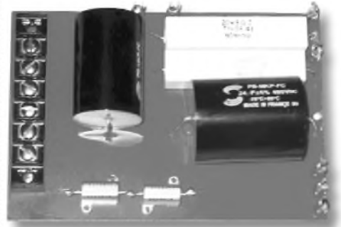
PHOTO 2: Component side of crossover board showing resistors, capacitors, and posts for connections to external components. (The series-connected resistors are a substitute for the specific parts, which were out of stock.)
