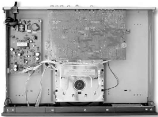
PHOTO 3: Inside the T550. The main PC board is mounted upside down. The switching power-supply board is on the left.
