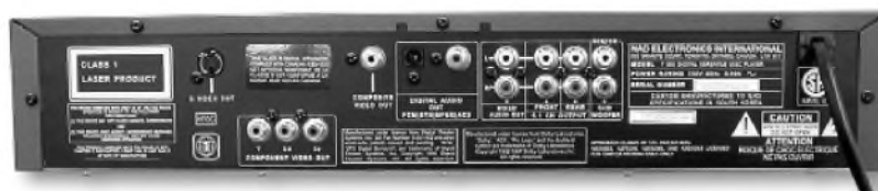
PHOTO 2: Rear panel of the T550. The player has built-in Dolby 5.1 decoding and the six required outputs. Separate stereo/mixdown outputs are provided for two-channel operation. Component, composite, and S-Video outputs are also included.
