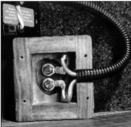
PHOTO 32: Attaching speaker leads.
