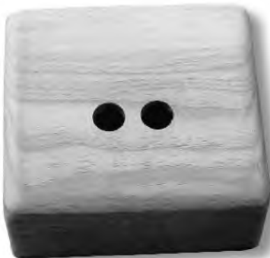
PHOTO 20: Terminal mounting block.
