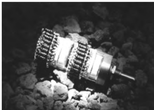
Picture showing a 4 layer 24-step stereo ladder type P&R attenuator
