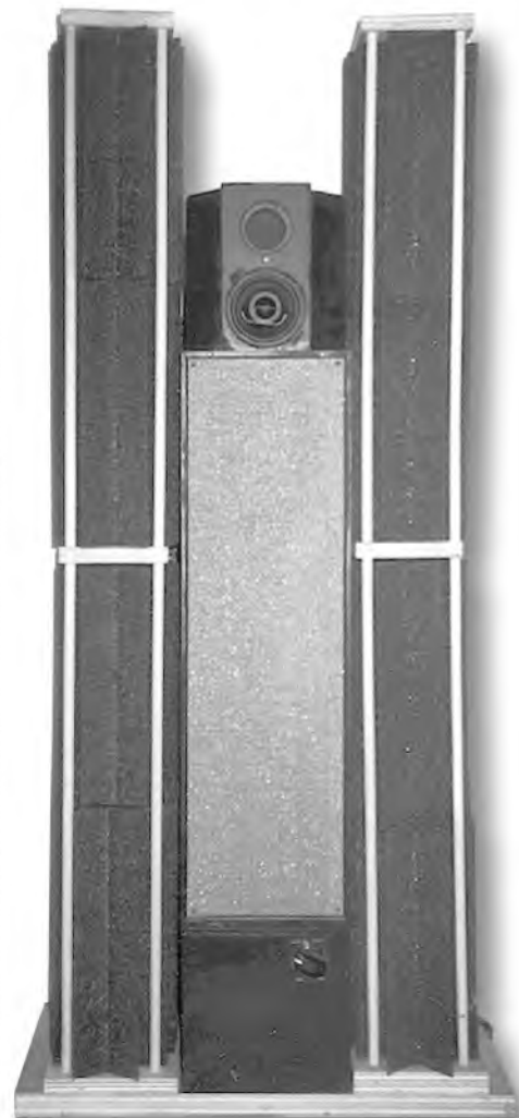
PHOTO 1: The revised left channel complete with absorbers. The treble unit is placed vertically and is flanked by 1.75"-thick blocks with 45° ends.
