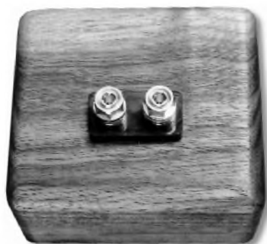
PHOTO 25: Finished terminal block.
