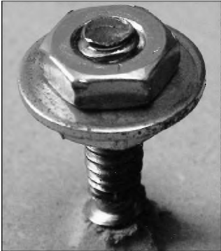
PHOTO 31: Mounting a hanger bolt.
