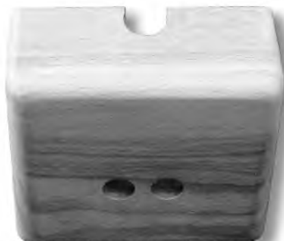
PHOTO 21: Slot for lead wires.
