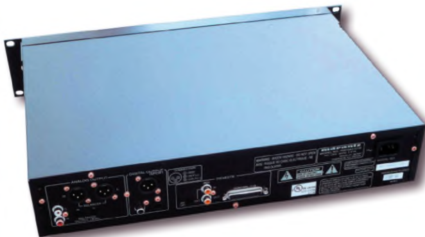
PHOTO 2: Rear view of the PMD340. This top-of-the line player in Marantz's current professional series has three digital outputs, along with both balanced and unbalanced analog outputs.
