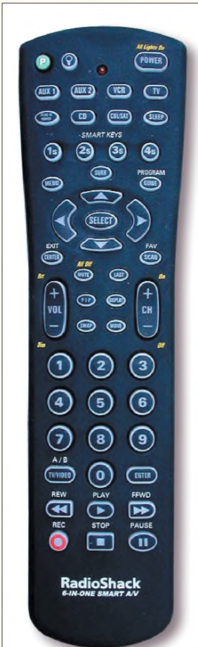
PHOTO A: The Radio Shack 15-1994 6-in-1 Smart A/V Remote. Compatibility with a wide variety of equipment, lack of directionality, and four learning buttons make this inexpensive remote a winner.
