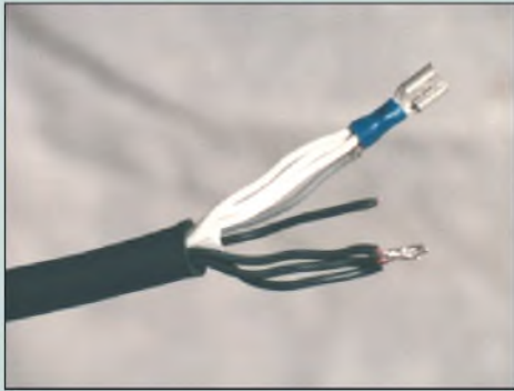
PHOTO 6: Short wires on woofer connector broke off, longer wires pulled free of the crimp. Note lack of solder on longer wires.
