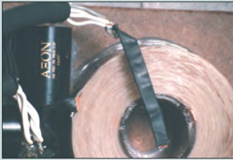
PHOTO 5: Note shiny copper foil just outside the coil bobbin where inductor lead used to be attached. The strain of the large Axon cable attached to the other end caused it to fatigue and break.
