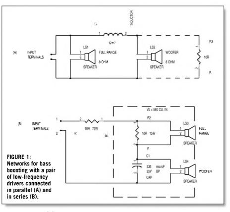
comprises a first-order low-pass filter network connected in parallel with LS1 to the input terminals of the speaker system. Resistor R3 is optionally connected in parallel with LS2. The first and second input terminals of LS1 and LS2 are positive and negative, respectively.
