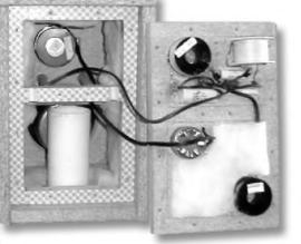
PHOTO 4: CSA front panel damping and crossover layout.
