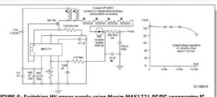
FIGURE 6: Switching HV power supply using Maxim MAX1771 DC/DC upconverter IC with Cooper voltage boost transformer.
