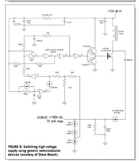
this circuit, although it does appear to be designed for maximum efficiency (possibly to provide high voltage for a vacuum-fluorescent display in a batterypowered device).
