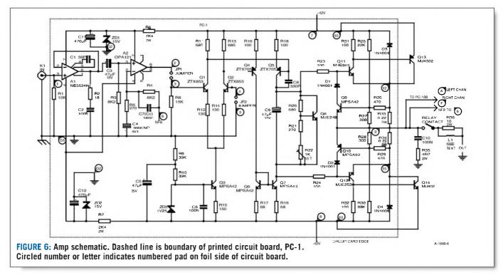
the best low-noise performance.<sup>3</sup> I would prefer it to be about an octave lower. Normally, it is possible to restrict bandwidth by using a small capacitor across the feedback resistor, but in this composite that space is already occupied by Cf. So I added a unity-gain, low-pass, active filter ahead of the composite.
