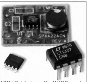
PHOTO 1: Clockwise from top: Sipex SP4422 IC mounted on Sipex evaluation board; Linear LT1307 switchingsupply IC; IMP803LG EL-lamp IC.
