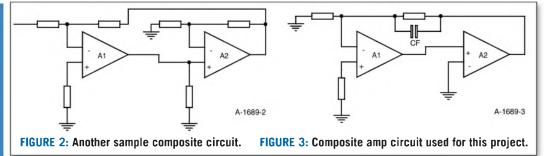
As things worked out, 2MHz was the highest unity-gain frequency I could achieve in A2 while still meeting the phase-margin requirements. All that's needed now to complete the composite is a compensated IC op-amp having an  $F_T$  of 2MHz. For this, I selected the OPA-121. Since this project is a power amp, you must also consider slew-rate needs.
