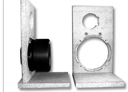
PHOTO 5: CSB front panel/bottom board assembly.
