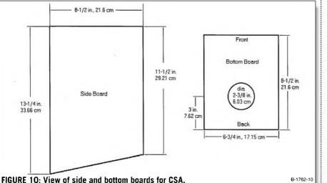
boxes. Install a 6"  $(15.24 \text{ cm}) \times 17$ " (43.18 cm) piece of nominal  $\frac{1}{2}$ " (1.27 cm) fiberglass, covering the bottom half of both sides and the bottom, cutting a hole to clear the port duct. Now glue the port ducts into the boxes flush with the bottom board.
