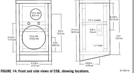
front-to-back dowels has holes (1/2" [1.27cm]) for the dowels and also notch. these notches with their outer end
