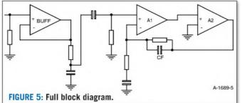
The intended output power is 50W into  $8\Omega$  up to 20kHz, which requires a minimum slew rate of  $3.55V/\mu s.^2$  The OPA-121 has a slew rate of 2V/ $\mu s$ . The composite solves the apparent slew rate shortage of this op-amp because it is multiplied by the gain of A2, as mentioned previously. The voltage gain of A2 at 20kHz is about 130, so the effective slew rate of A1 is 260V/ $\mu s$ .
