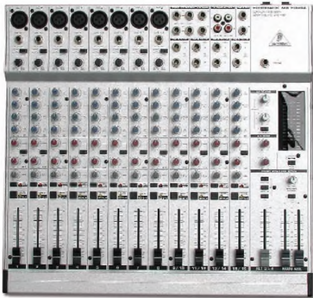
PHOTO 2: Behringer MX2004A mixer. Up to 20 inputs, and considerable flexibility are offered in this fine performer. The logarithmic input and output faders feature a 60mm travel.
