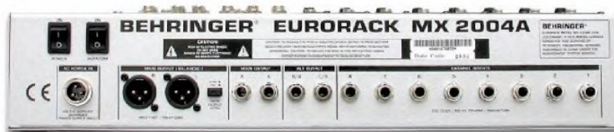
PHOTO 3: Behringer MX2004A rear panel. The XLR main outputs can be switched from line to mike level. Channel inserts for the eight mono inputs, 1/4" main outputs, and the Alt 3 and 4 outputs are on the rear panel.
