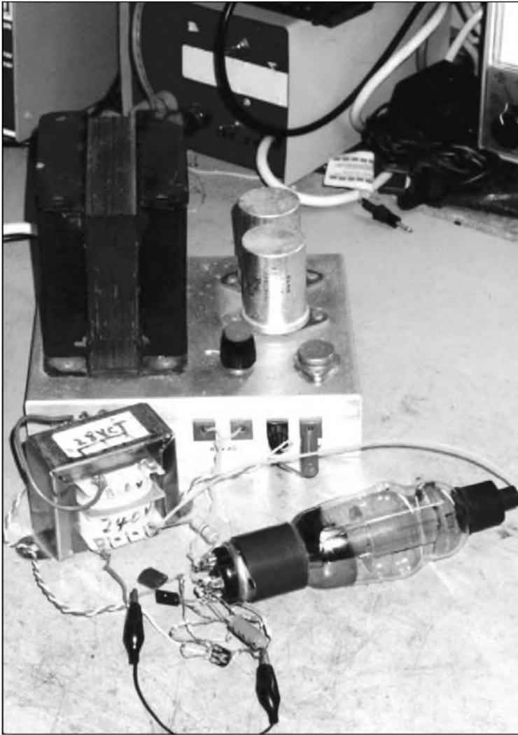
PHOTO 2: My test setup, with power supply, output transformer, and circuitry.
