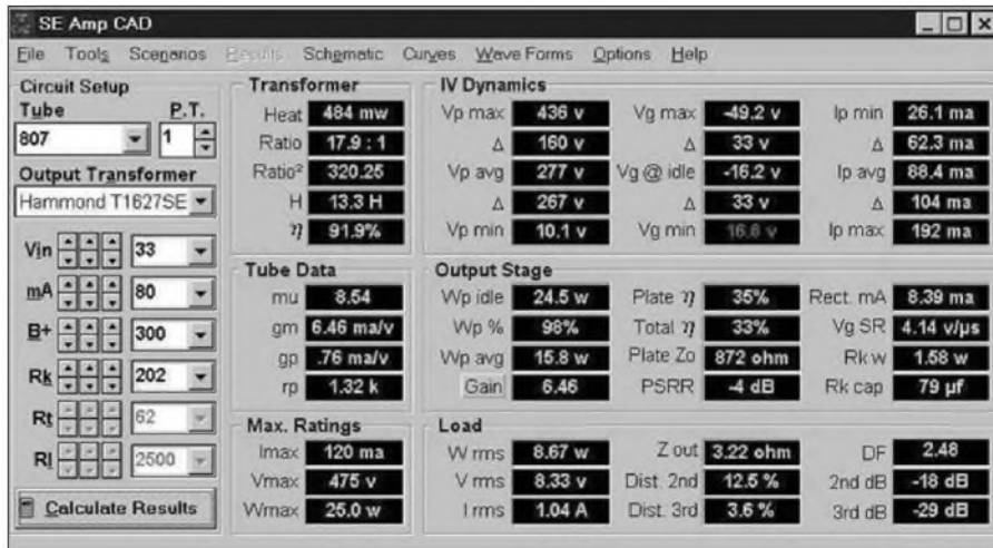
FIGURE 15: Prototyping experimental tube circuits with SE Amp CAD.
