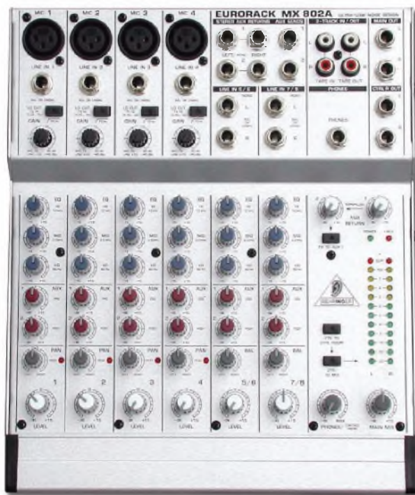
PHOTO 1: Behringer MX802A mixer. The compact design still offers a wide array of features and excellent performance. All audio input and output connectors are on the mixer top plate, as shown.
