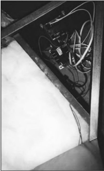
PHOTO 7: An overhead view showing the woofer area (stuffed), the rear woofer deflector, and the electronics area.
