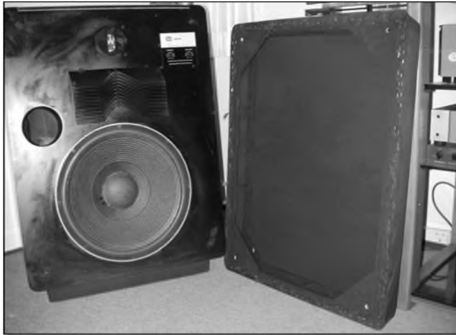
PHOTO 2: Prior to rebuilding the grille.
