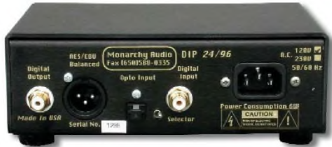
PHOTO 4: Rear view of the DIP 24/96. Both coax and Toslink optical inputs are included, along with coax S/PDIF and AES/EBU outputs.
