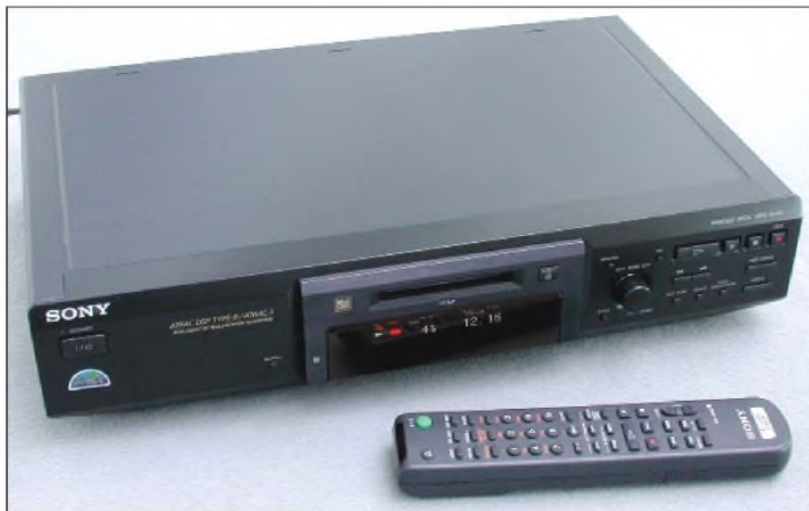
PHOTO 1: The Sony MDS-JE440 MiniDisc Deck and supplied remote control. This entry-level component MiniDisc recorder is intended for use with a complete audio system, and matches the styling of Sony's CDP-XE400 and XE500 CD players.
