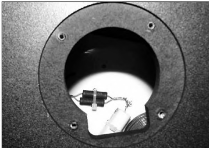
PHOTO 9: Crossover mounting screw visible through tweeter opening.
