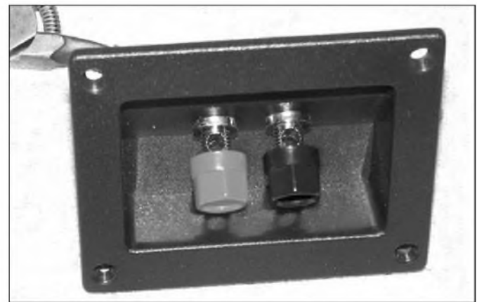
PHOTO 6: Proper alignment of binding posts.
