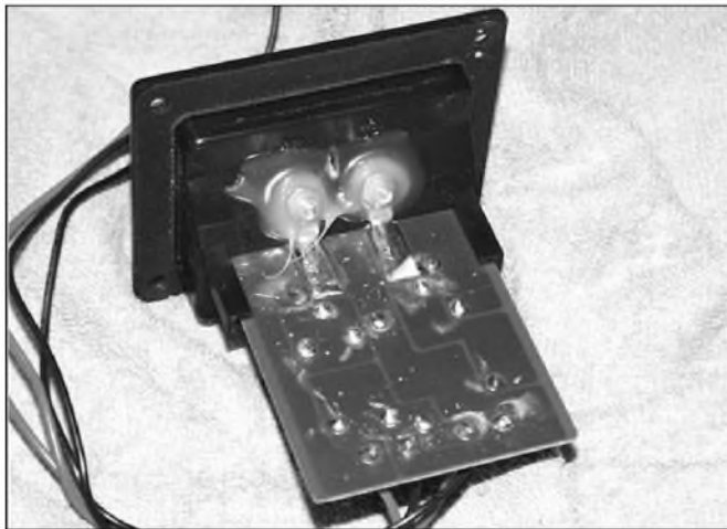
PHOTO 4: Binding post plate—as received.
