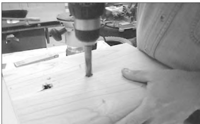
PHOTO 24: Drilling holes in the laminate to trim the driver holes.
