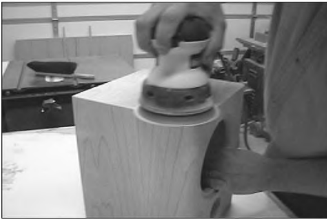
PHOTO 26: Sanding the laminate.
