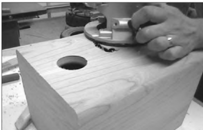
PHOTO 25: Trimming the driver holes.
