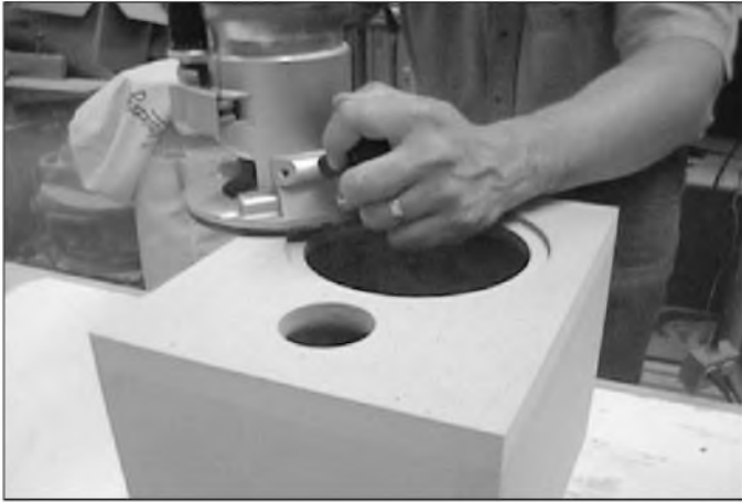
PHOTO 18: Routing a round-over on the side edges of the front.
