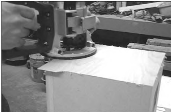
PHOTO 23: Using a laminate trimmer to trim the top veneer.
