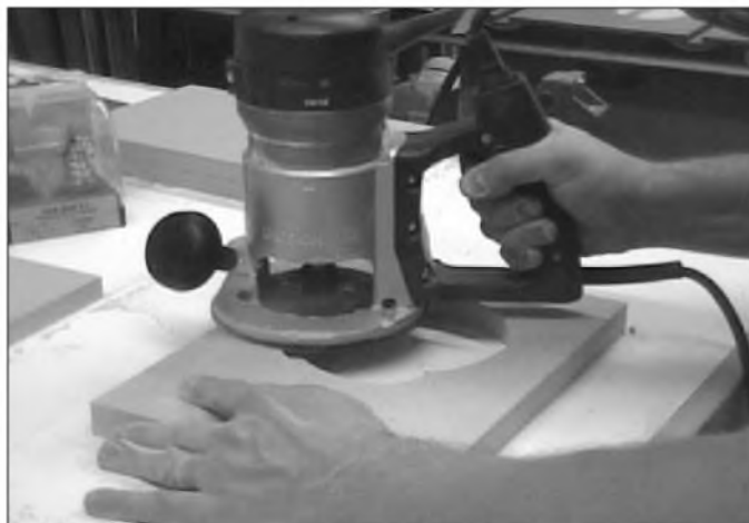
PHOTO 9: Routing the driver recess.
