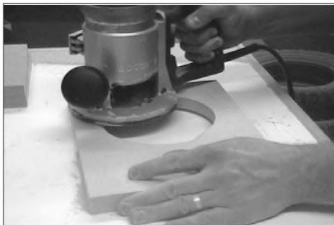
PHOTO 10: Routing the round-over on the back of the driver hole.
