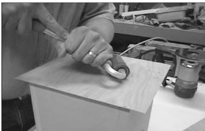
PHOTO 22: Using a J-roller to apply pressure to the veneer.
