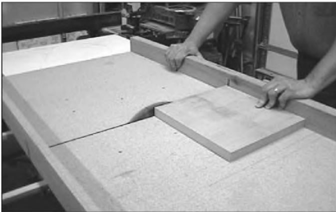
PHOTO 2: Squaring up the reference corner with a crosscut sled.
