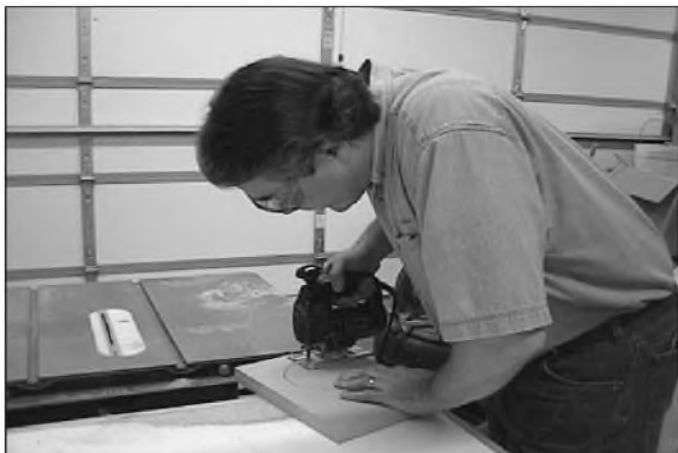
PHOTO 7: Cutting out a driver hole with a jig saw.
