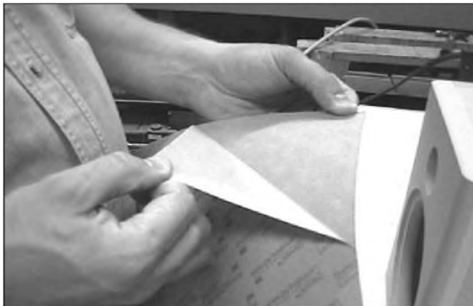
PHOTO 20: Peeling veneer backing.
