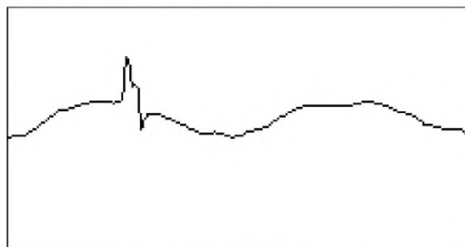
FIGURE 7: A click in a periodic waveform.
