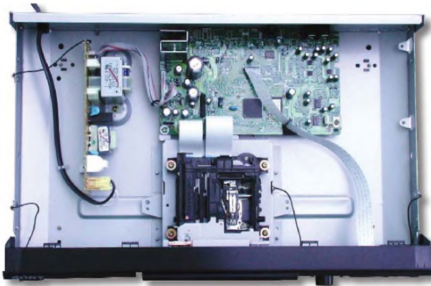
PHOTO 3: Inside the MDS-JE440. A handful of proprietary Sony chips make up most of the circuitry.
