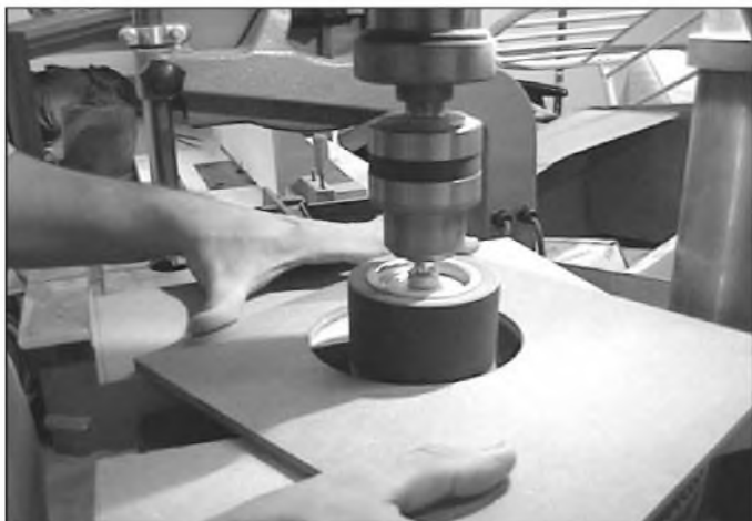
PHOTO 6: Sanding the template with the drum sander.
