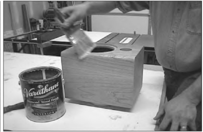
PHOTO 27: Applying urethane finish.
