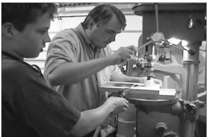
PHOTO 5: Cutting a tweeter hole with a hole saw.
