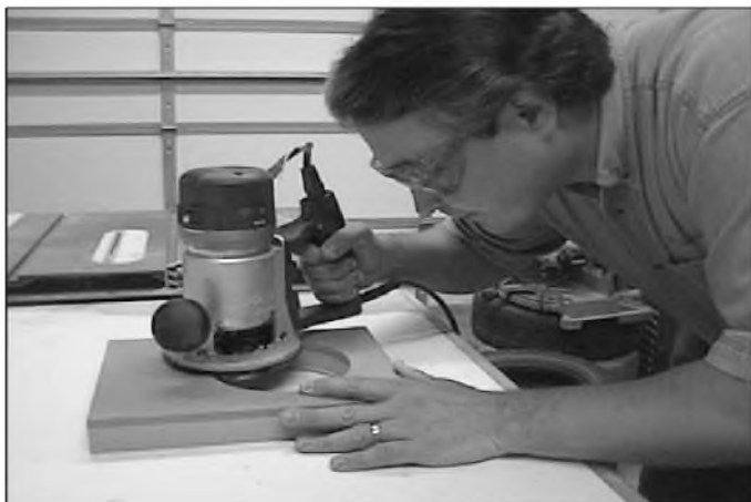
PHOTO 8: Routing a driver hole with a template.
