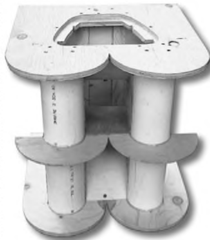
PHOTO 15: The halved PVC in place.
