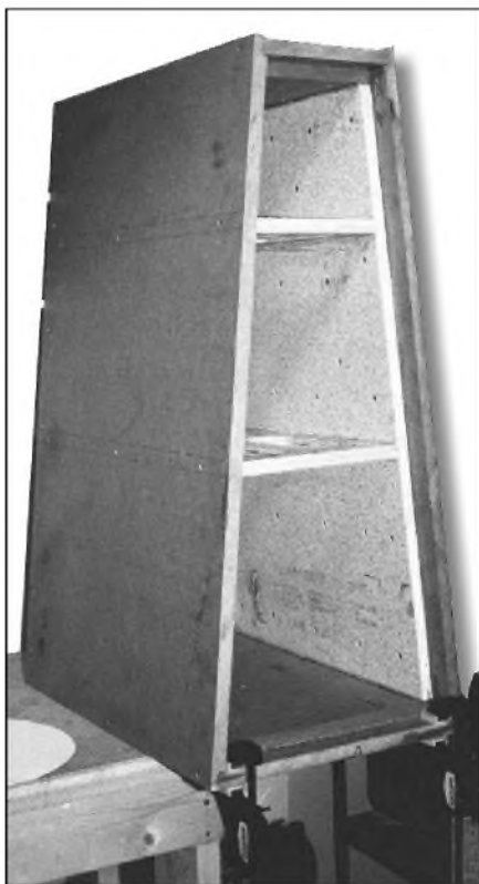
PHOTO 8: Assembled bass cabinet, prior to front baffle installation. Note horizontal braces used on prototype not necessarily recommended (see text and drawing).
