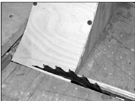
PHOTO 5: Trimming the throat horn on a cutting jig.
