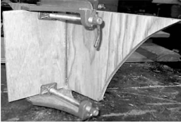
PHOTO 2: The throat-horn divider clamped to throat-horn side.
