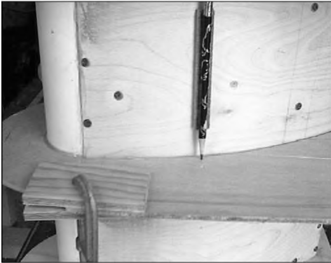
PHOTO 16: Attaching the side braces.
