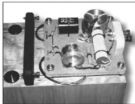
PHOTO 7: Top view of bass cabinet with crossover mounted.
