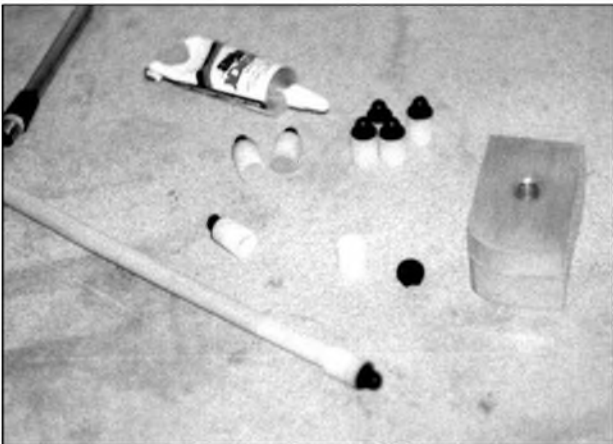
PHOTO 20: Aluminum block for sanding stand-off mounts.
