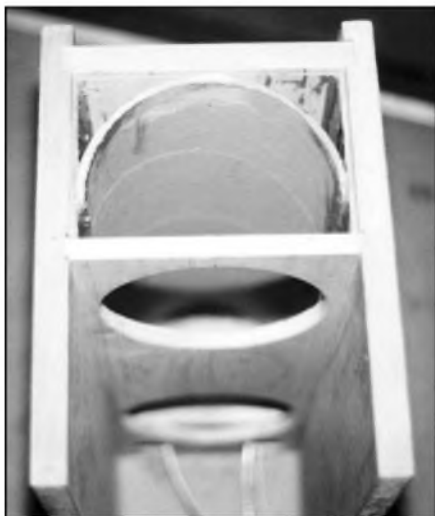
PHOTO 14: Open view of top of satellite showing half section of cardboard tube. "Dead" back corners to be sand-filled.
