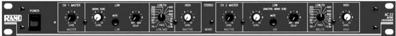
PHOTO 1: AC 22 front panel. From left to right: on/off switch, power indicator, master input gain, low-pass gain, low-pass mute switch, delay control, crossover frequency selector, and high-pass gain. Repeated for the second channel.
