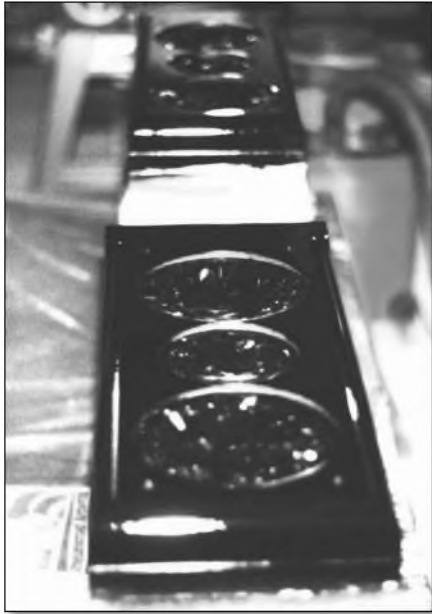
PHOTO 19: Painting satellite fronts.
