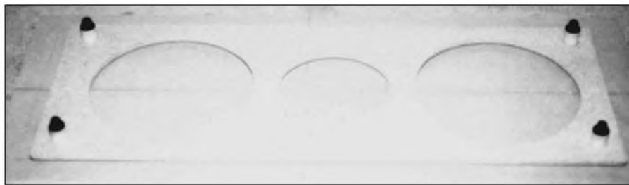
PHOTO 21: Back side of stand-off grille, showing mounts.
