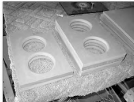
PHOTO 10: Finished braces. Top braces on left.
