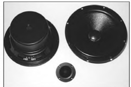
PHOTO 27: The drivers—Adire AV8 midwoofers (2) and an Audax tweeter.
