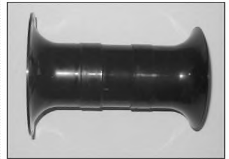
PHOTO 20: The flared port, cut to length and glued together.
