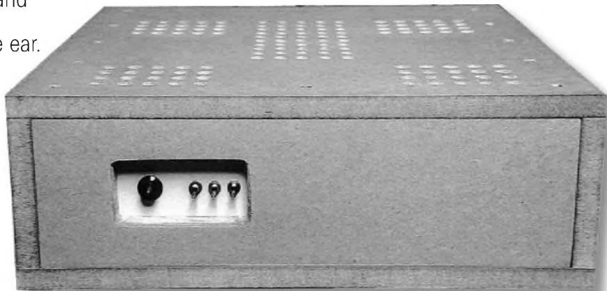
PHOTO 1: Front view panel showing a neon mains-on lamp, sided by three double-pole switches: mains on/off, filament on/off, and H.V. on/off, respectively.
