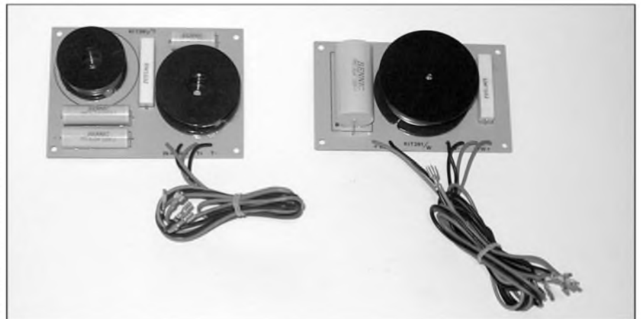
PHOTO 21: The crossovers, as supplied. HF is on left, LF on right.
