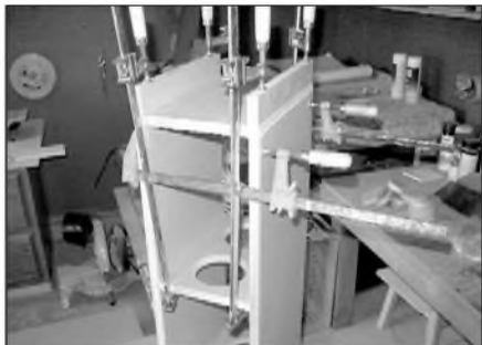
PHOTO 13: Gluing on the top. The bottom is done the same way.
