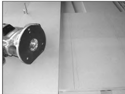
PHOTO 4: Setup to cut straight dadoes in sides, two at one time.
