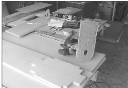
PHOTO 8: Router with circle jig, preparing to cut round holes in brace.
