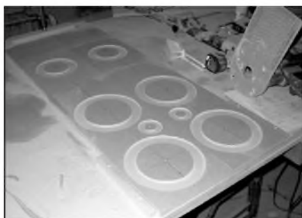
PHOTO 9: Circular dadoes in the two front panels are cut before the circular holes.
