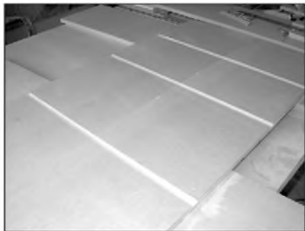
PHOTO 6: Sides with completed dadoes.
