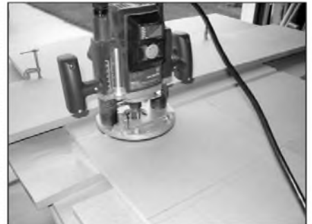
PHOTO 5: Cutting straight dadoes in sides two at a time.
