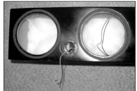
PHOTO 26: Stuffing the box. Wires from crossovers are routed to the driver cutouts.
