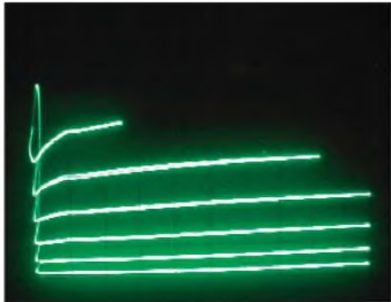
FIGURE 7: VacuTrace curves for matched EL34 "A" (sample #1).
