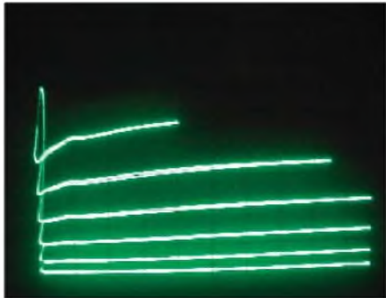
FIGURE 8: VacuTrace curves for matched EL34 "B" (sample #2).
