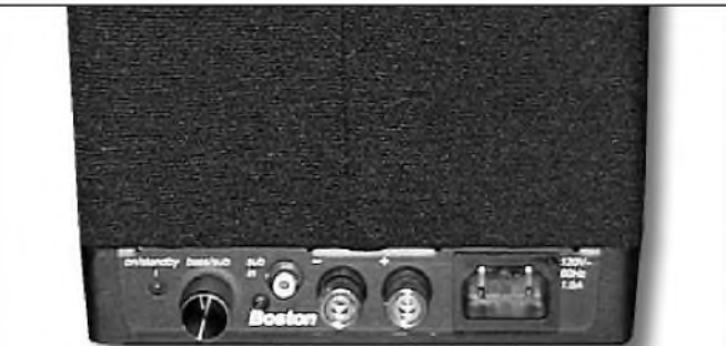
PHOTO 5: VR-975 input connections and subwoofer control.
