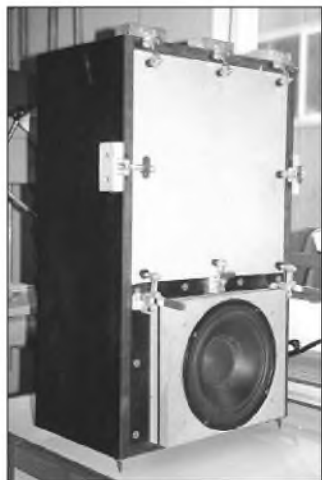
PHOTO 4: Woofer panel “floating” on \frac{1}{4} " neoprene damping layer.
