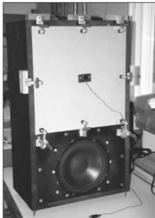
PHOTO 2: Test panel in place with ACH-01 accelerometer fastened with double-stick tape.
