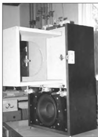
PHOTO 3: External cabinet with single large oval brace with 1" frames.
