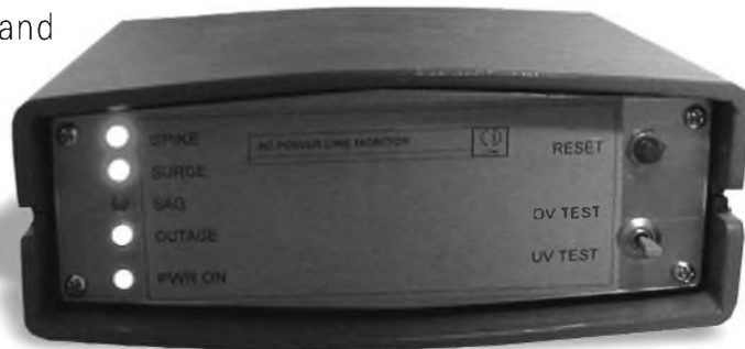
PHOTO 1: Power line monitor.
